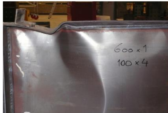
FIGURE 44: GIRDER NUMBER 7, TESTED BY ABSPOEL WITH A WEB-SLENDERNESS OF 600
