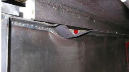
FIGURE 43: GIRDER NUMBER 4 TESTED BY ABSPOEL, WITH A WEB-SLENDERNESS OF 400
