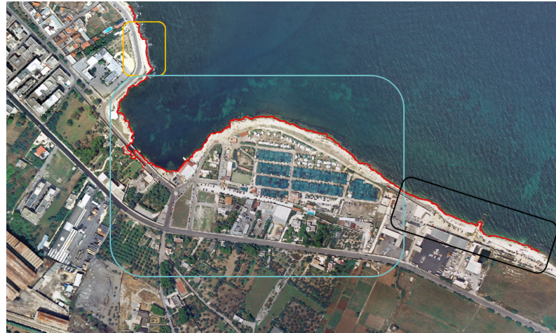
Figure 11. Example of the shoreline extracted along Apulian beaches overlapped on ortho-images. The yellow box delimits the breakwaters zones, the blue box marks the rocky beaches and the black box delimits sandy beaches limits.
