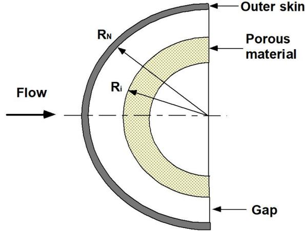
Figure 4-1: Configuration of Enhanced radiation cooling.
