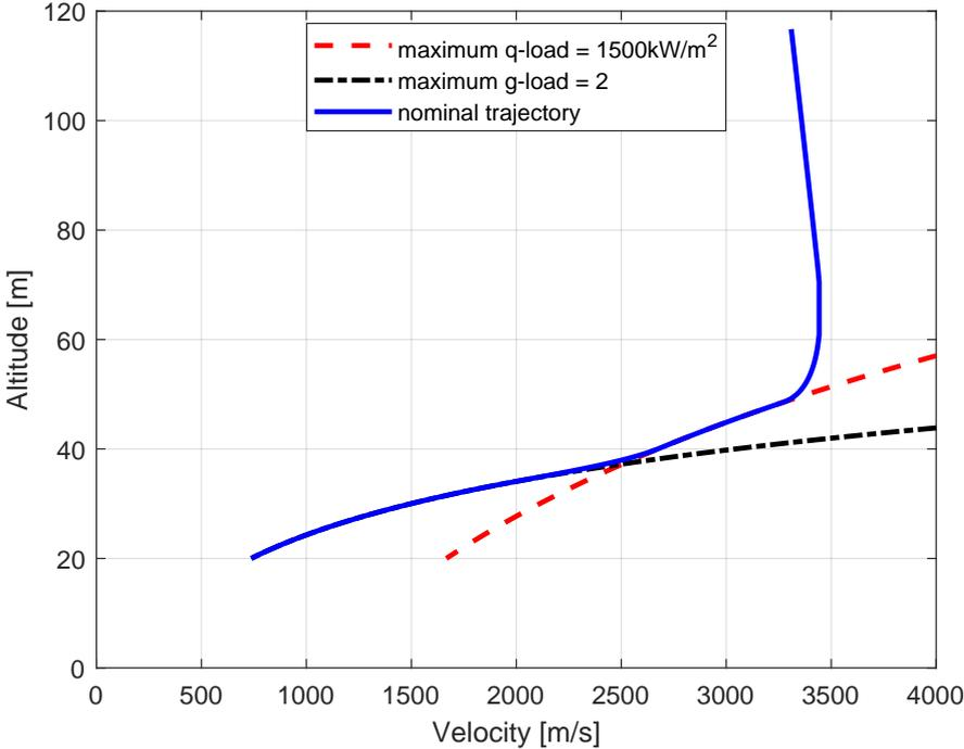
Figure 2-23: Altitude-velocity profile for nominal trajectory.
