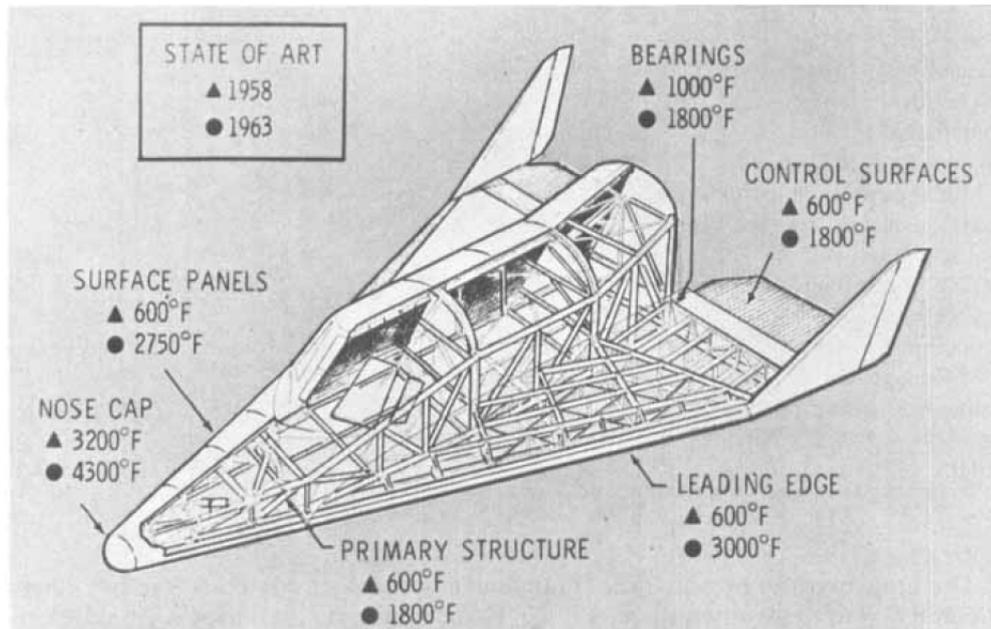
Figure 2-1: X-20 material temperatures (Rotelli, 1965).
