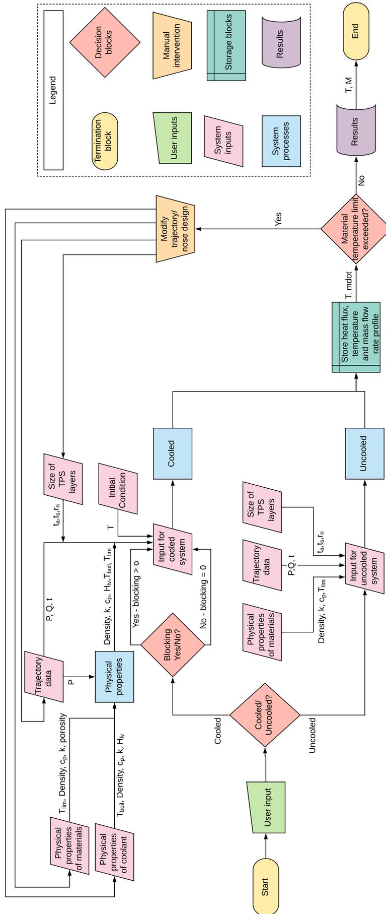
Figure 4-3: Flow chart for transient model.
