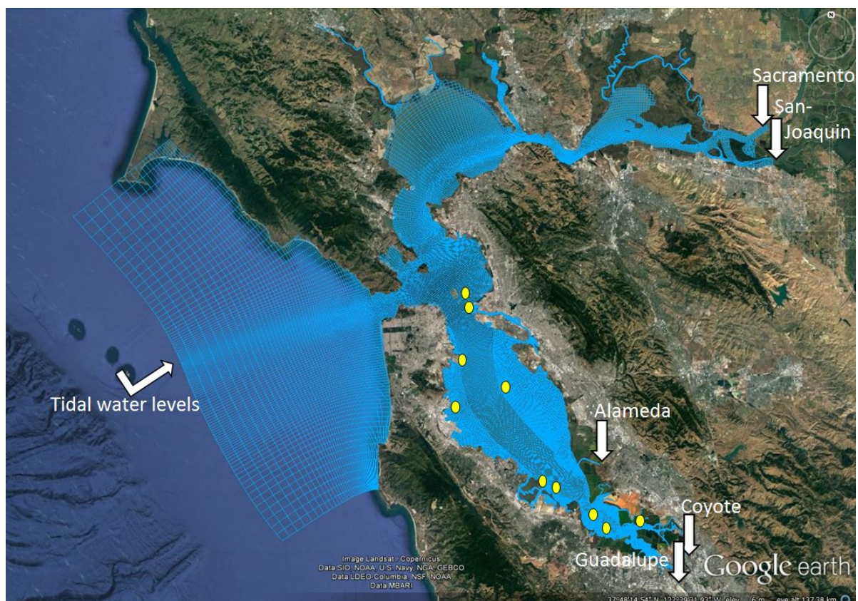
Figure 3.2: Model grid of D-Flow FM of San Francisco Bay is shown in blue. The model is driven by tidal water levels at the Pacific boundary and discharges at the five river boundaries, both displayed with the with arrows. The outflow locations of the waste-water treatment plants are shown with yellow dots.
