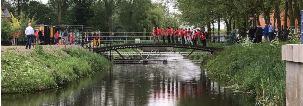
Fig. 28 Loadcase 2. Asymmetric load with 39 students; approx. 2.11 kN/m
