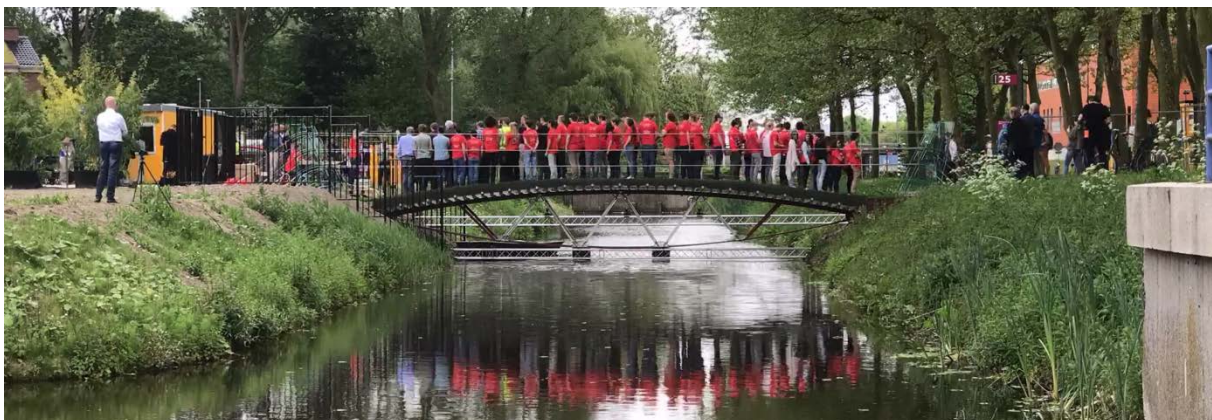
Fig. 27 load case 1. 67 students; approx. 1.81 kN/m
