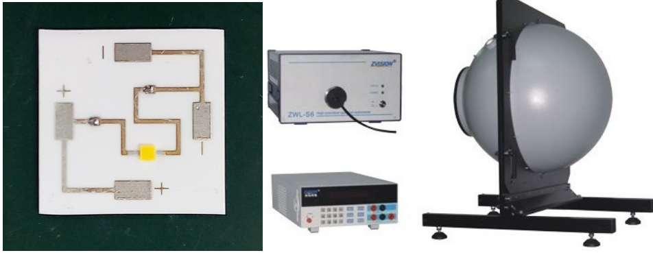
Figure 3.4: The LED Sample and the Integrating Sphere System.
