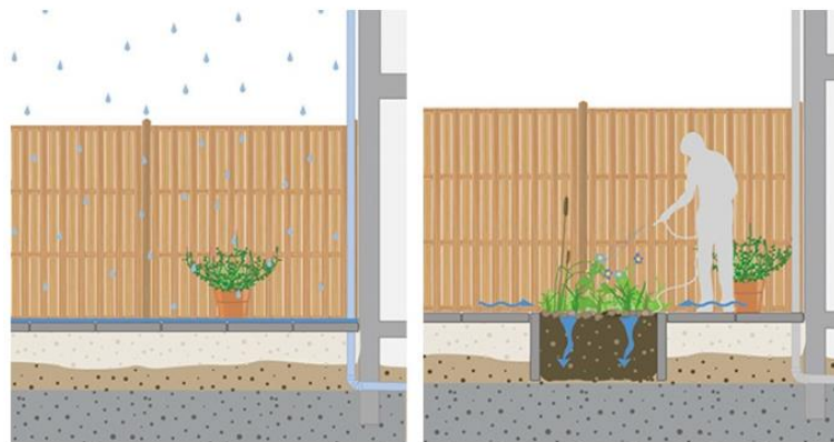
Figure 2.3: Impervious and pervious surfaces (Amsterdam Rainproof, n.d)
