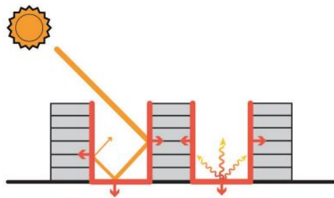
Figure 2.2: Heat trapping in street canyons (Pijpers-van Esch, 2015)
