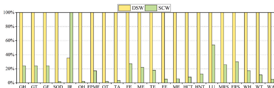
Fig. 14. The endpoint environmental impacts of 1 m 2 DSW and SCW by ReCiPe (2016) method.
