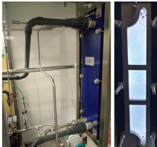
Figure 4.2: Pictures of the experimental setup (top), test section (bottom-left) and visualization section (bottom-right). In the top figure, the experimental setup consists of a GPHE (test section), three BPHEs (evaporator, recuperator, after cooler), two working fluid tanks (separator, buffer tank), two water tanks (cold water, hot water), a working fluid pump, four water pumps (cold water driven pump, cold water mixing pump, hot water driven pump, hot water mixing pump). In the bottom-left figure, the test section is shown before being wrapped with insulation materials. The inlet and outlet ports of \text{NH}_3 are connected with stainless steel tubes, while the inlet and outlet ports of \text{H}_2\text{O} are connected with PVC tubes. In the bottom-right figure, the visualization section is composed of a transparent end plate and a frame plate with three observation windows. It is illuminated by an LED-strip circumferentially.
