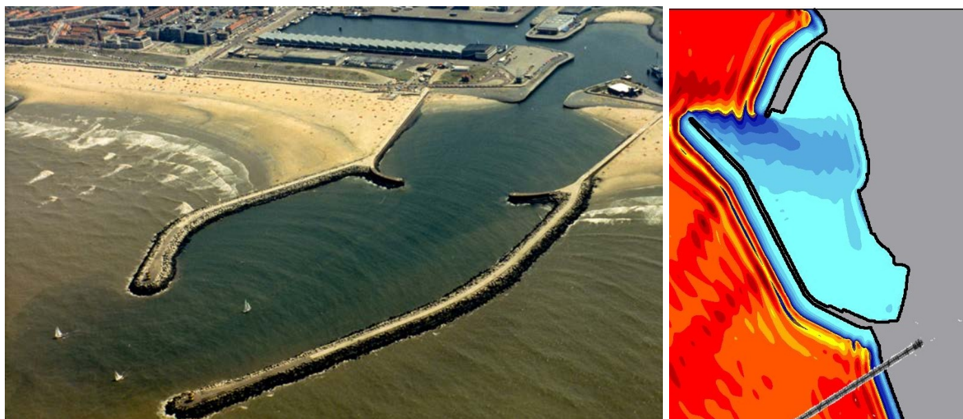
Figure 3.10: Left: wave penetration and diffraction in the Port of Scheveningen, the Netherlands ( http://beeldbank.rws.nl , Rijkswaterstaat ). Right: Boussinesq model results for Buchanan Port in Liberia to calculate wave penetration around breakwaters (by Royal HaskoningDHV is licensed under CC BY-NC-SA 4.0).
