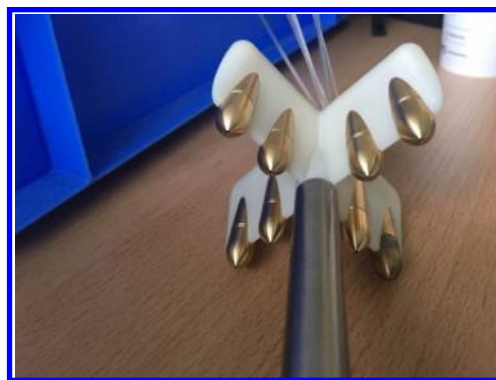
Fig. 3 HFSB rake with the 8 generators. The transparent capillaries carrying helium, soap and air can be seen in the back
