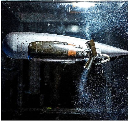
Fig. 4 Photograph of the TR model in the test section. The HFSB particle streaks are visible within the seeded jets.
