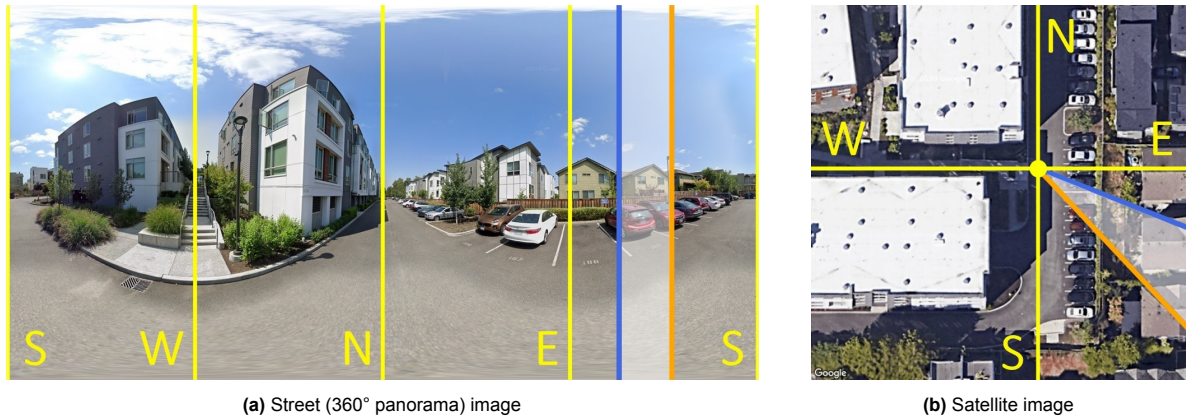
Figure 1.3: A street and satellite image pair that shows the azimuth prior, i.e., the geometric relationship that every vertical line in the street image has a corresponding azimuth direction in the satellite image. The yellow dot indicates the street camera location in the satellite image, and the yellow lines indicate the compass strokes. Both the blue and the orange lines show an azimuth direction. These two lines delineate a slice in both images, i.e., the transparent region. The street image slice and the satellite image slice belong to each other and have a visual overlap. The image pair is part of the VIGOR dataset [107].
