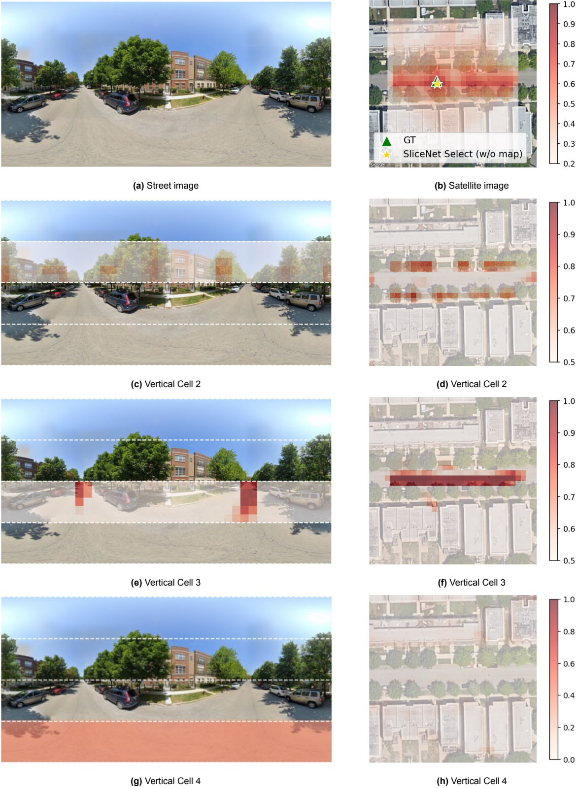
Figure 4.8: Image pair 2 with the corresponding similarity map in overlay on the satellite image and the attention maps. The model that has been used is SliceNet Select (w/o matching map) with eight horizontal slices and four vertical cells. All street attention maps use the same color bar as the satellite attention maps. The image pair is aligned. The images are part of the test split of Chicago (same-area) of the VIGOR dataset [107].
