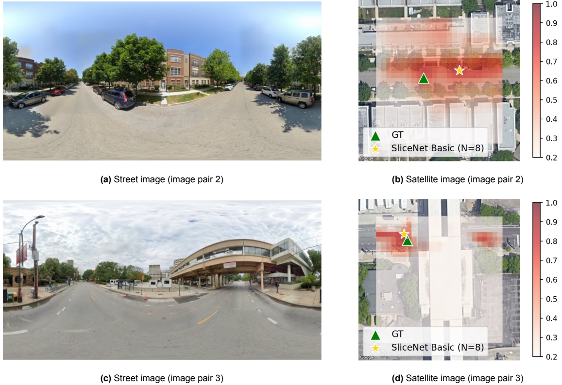
Figure 4.5: Image pairs 2 and 3 with the corresponding similarity map in overlay on the satellite image. SliceNet Basic ( pose loss ) with eight horizontal slices has been used. All image pairs are aligned. The images are part of the test split of Chicago (same-area) of the VIGOR dataset [107].
