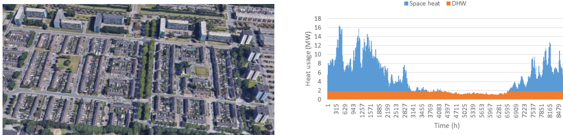
Fig. 2. District Biesdonk in Breda selected for implementation of the LTDH designs (left) and heating requirement for 650 terraced houses and 1000 apartments in 2016 (right).
