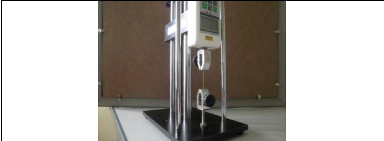
Fig. 7 Root is pulled by a digital force gauge
