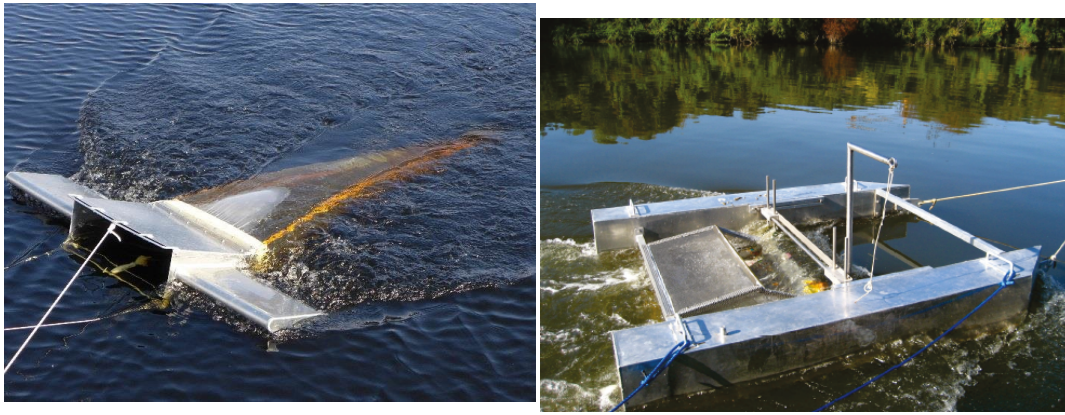
Figure A.1: A manta net sampler. Photo by Julia Farkas, SINTEF Ocean. Figure A.2: A WFW-sampler.
