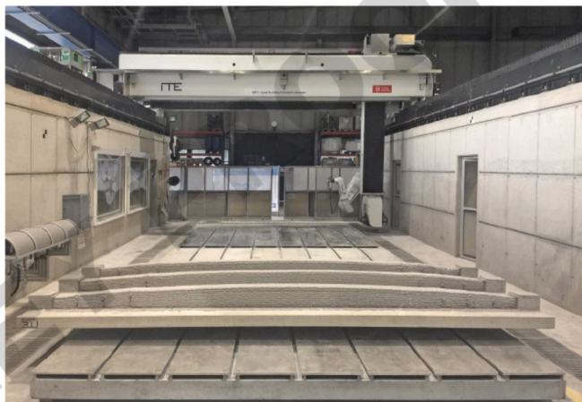
Fig. 9. Add-on Printing of (a) concrete ribs with varying cross-section height according to the course of the bending moment [29].
