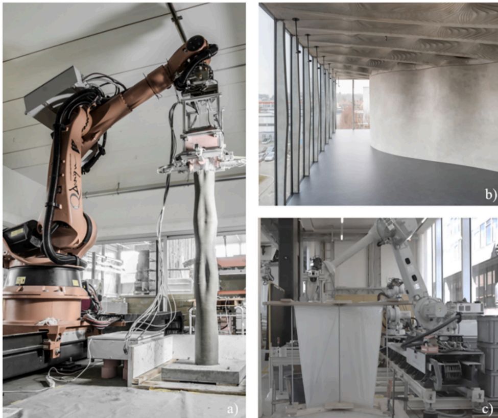
Fig. 21. a) Smart Dynamic Casting: Robotic Slipforming with flexible formwork [78], b) DFAB House, image Gramazio Kohler Research [80], c) ACDC Supported Thin Formwork [69].
