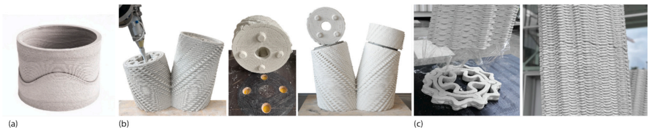
Fig. 4. Assembly interfaces for segmented columns (Digital Building Technologies ETH Zurich): (a) Vertical stacking of non-planar layers with variable layer height [8]; (b) 3D Printed branching columns: Incremental rotation of layers to align layers to main loads [25]; (c) Tor Alva - match casting for segmental assembly [25].
