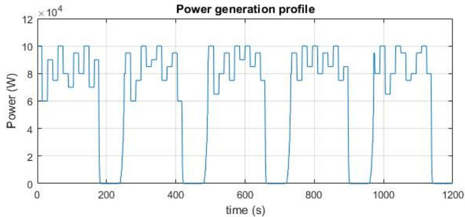
Figure 5.7: *KP system power generation profile*
