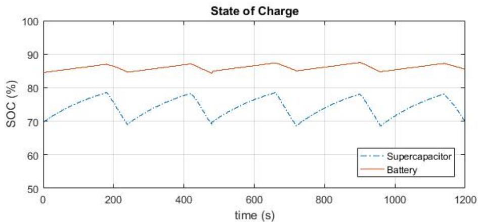
Figure 5.6: State of charge of the supercapacitor and Battery
