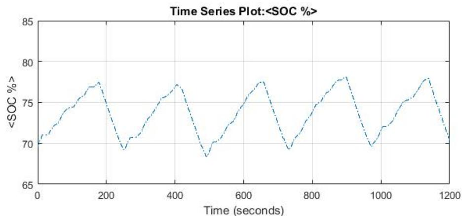
Figure 5.10: State of charge of the KP system supercapacitor
