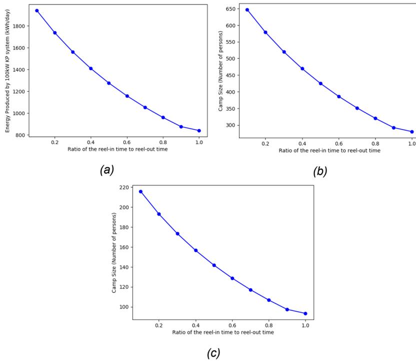
**Figure A.1: Energy produced depending on the reel-in to reel-out time ratio, with 30% of the power produced needed for the reel-in phase. b) Camp size with a consumption of 3kWh/day per person. c) Camp size with a consumption of 9kWh/day per person**
