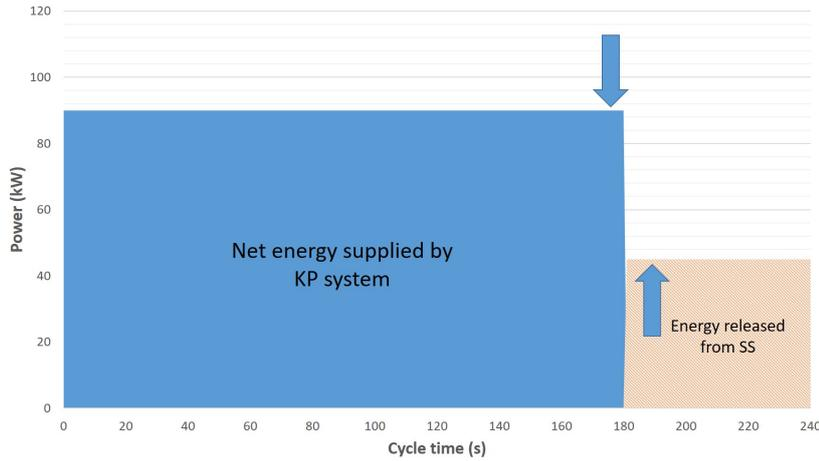
Figure 3.1: Example of the energy distribution of an AWE system with SS
