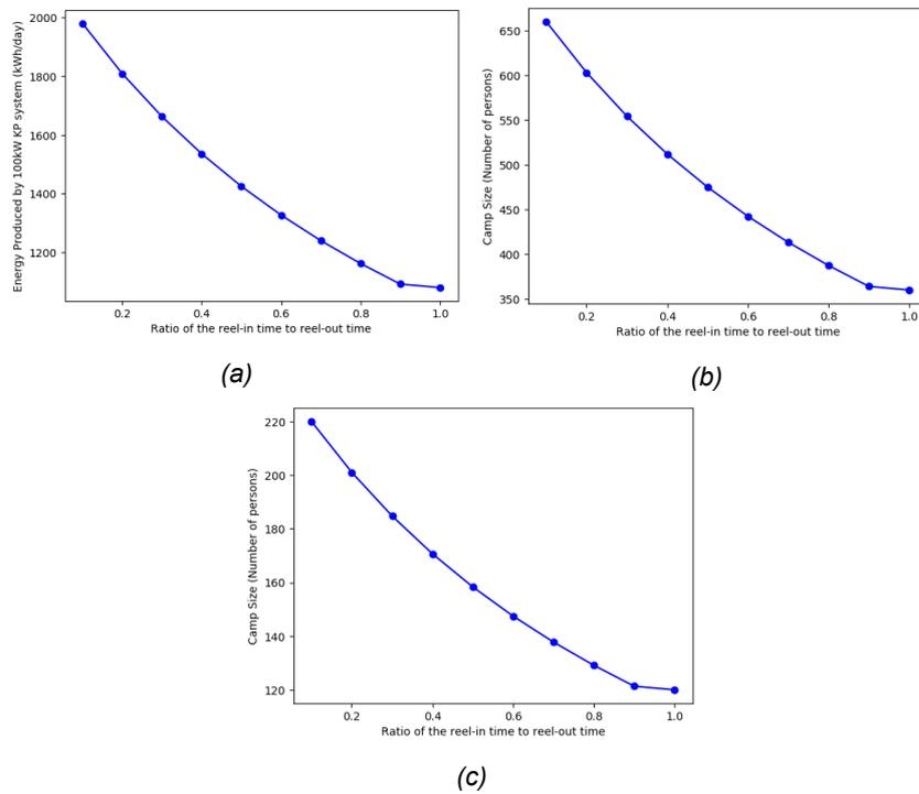
**Figure A.3:** Energy produced depending on the reel-in to reel-out time ratio, with 10% of the power produced needed for the reel-in phase. b) Camp size with a consumption of 3kWh/day per person. c) Camp size with a consumption of 9kWh/day per person
