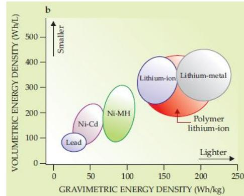
**Figure 2.3: Comparison of the energy store capacity between rechargeable batteries [12]**
