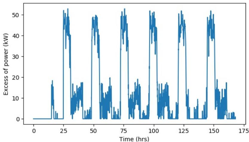
Figure 5.15: *Excess of energy produce by a KP system giving 59 kW*
