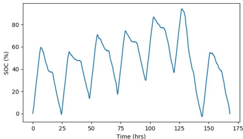
Figure 5.14: **State of Charge of the 345kWh battery**
