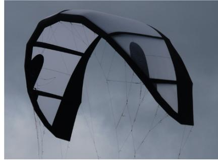
Figure 1.1: **Leading Edge Inflatable kite of KitePower** (Source: <http://www.kitepower.eu>)
