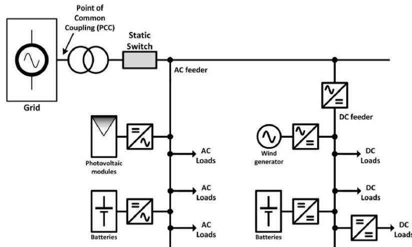
Figure 1.7: Hybrid AC/DC microgrid[18]
