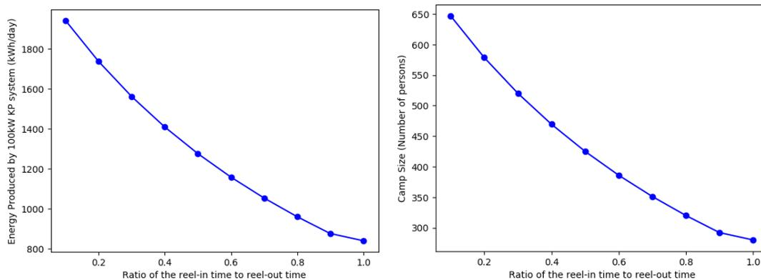
**Figure 5.1: Energy produced and camp size depending on the reel-in to reel-out time ratio. With 30% of the power produced needed for the reel-in phase and a consumption of 3kWh per person**
