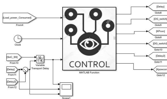
Figure D.2: KP generator simulink model
