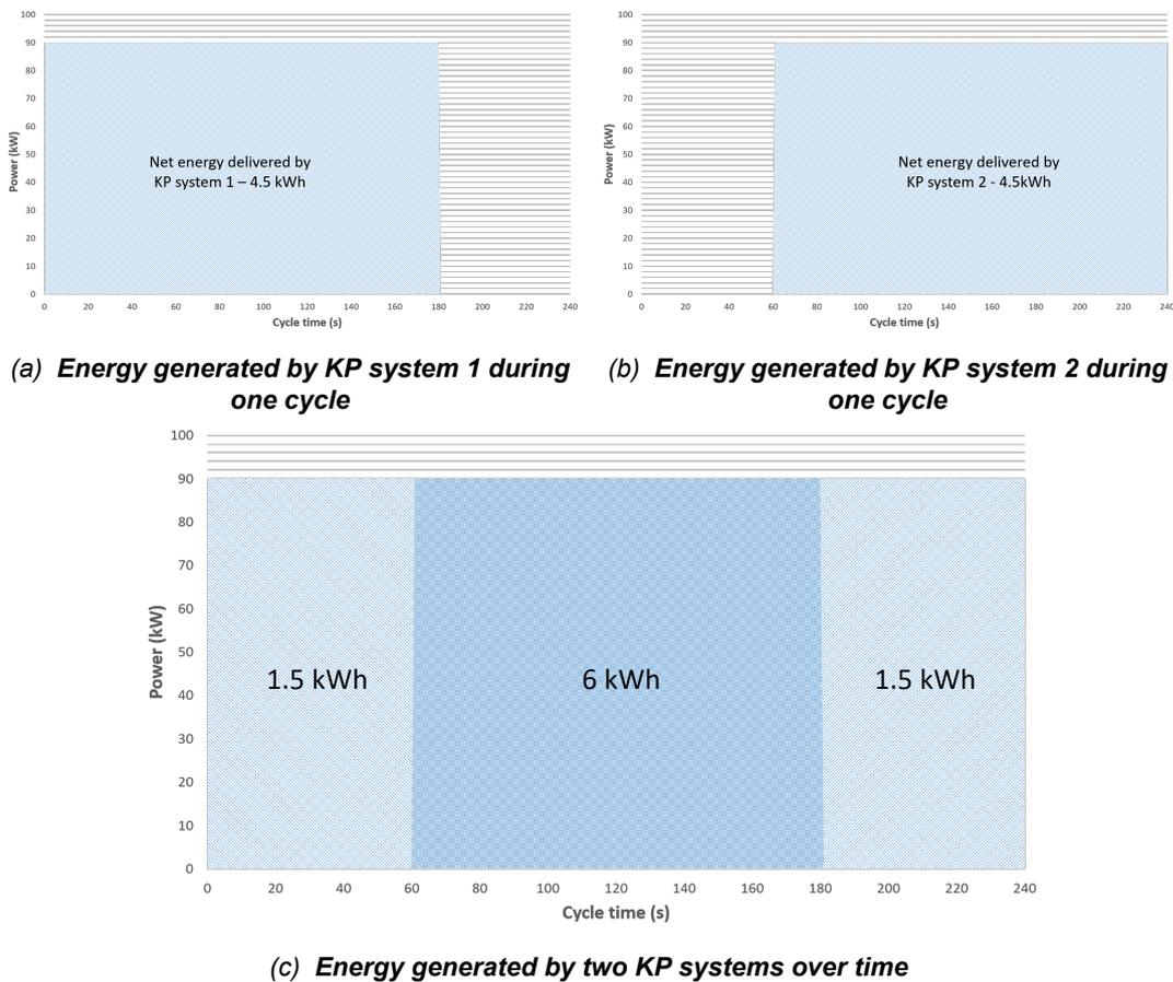
Figure 2.2: Energy distribution of 2 synchronized KP system with an optimum reel-out time
