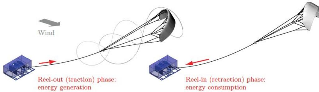
Figure 1.2: Pumping Cycle Kite Power operation [7]
