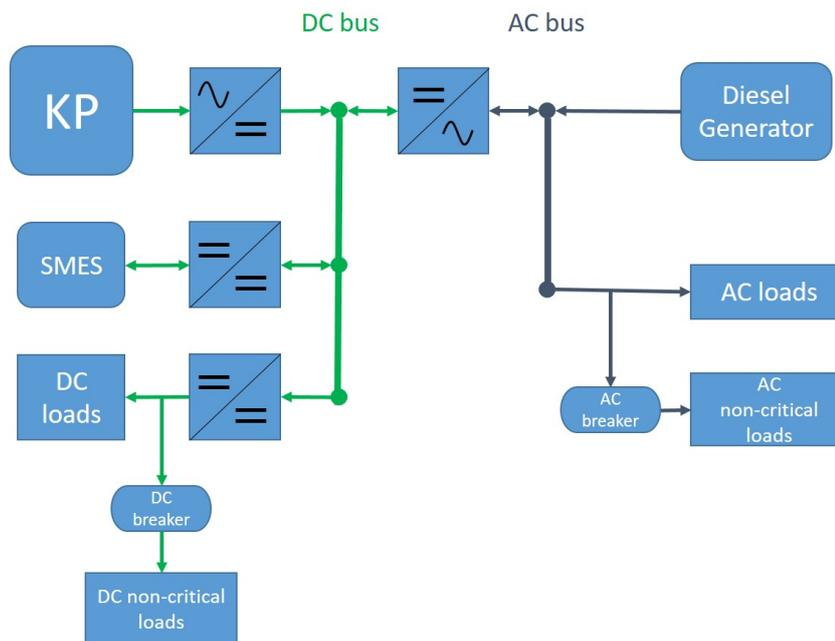
Figure 4.1: **AWE microgrid configuration with hybrid DC and AC bus**
