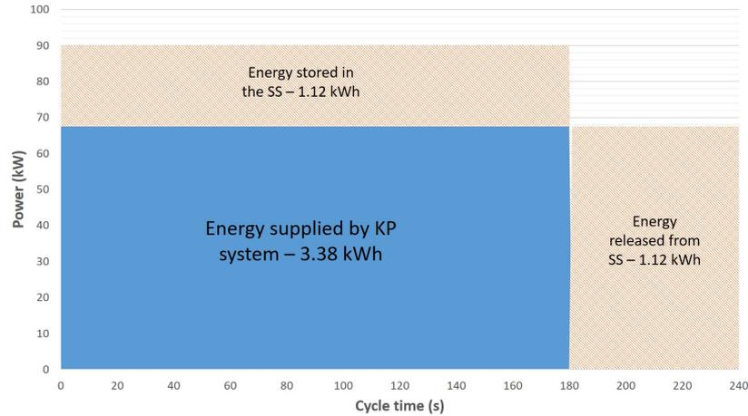
Figure 5.2: Energy supplied profile for the microgrid
