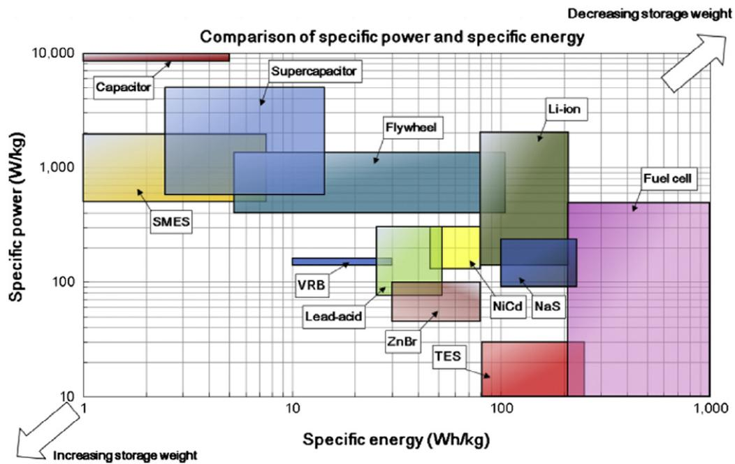
Figure 2.6: Specific power and specific energy of the most common SS[24]
