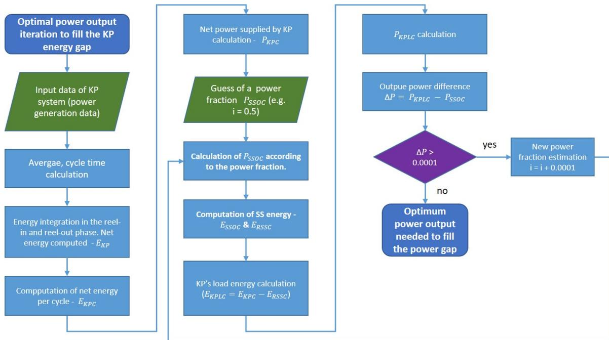
Figure 3.2: Iteration flow chart used to find the optimal SS power output to fill the power gap
