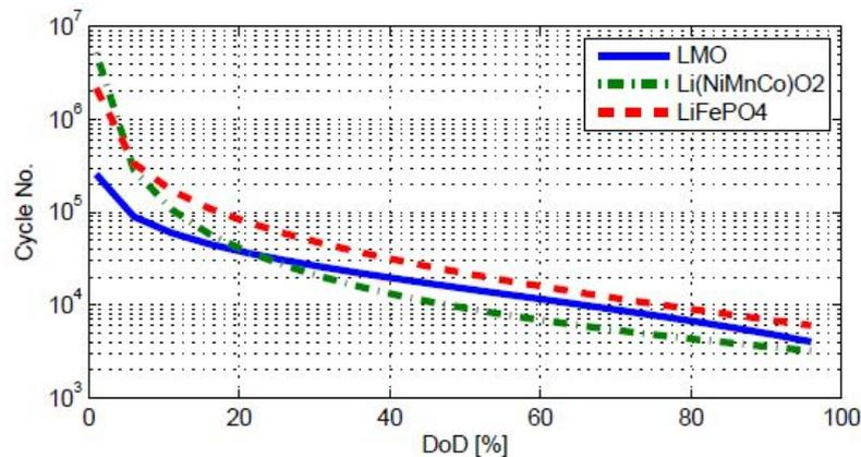
**Figure 2.4: Number of Cycles according to the DOD of a Lithium-ion battery [14]**
