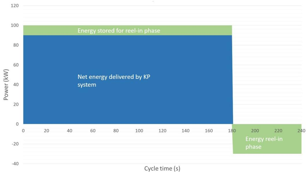
Figure 2.1: *Hypothetic energy distribution of one cycle of an AWE system*
