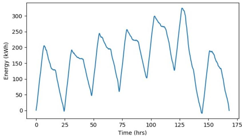
Figure 5.13: **Energy flow of 100 households in summer with a constant production power of 46.9kW**
