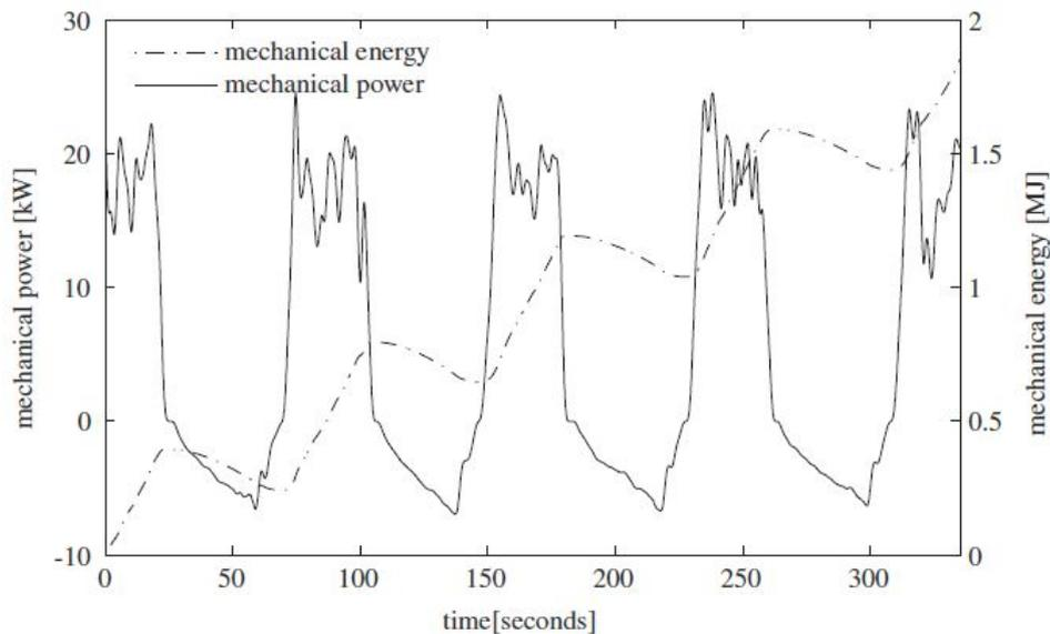
Figure 1.3: Traction power and mechanical energy over four pumping cycles [2]
