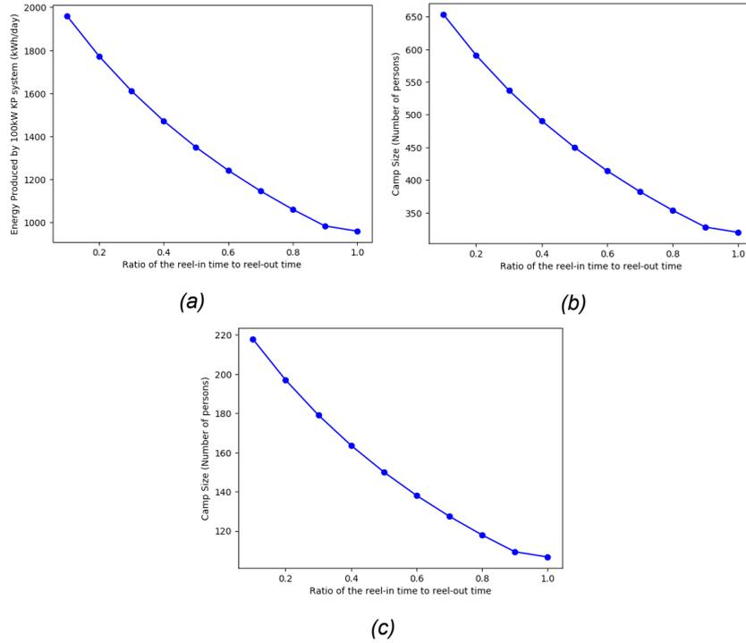
**Figure A.2:** Energy produced depending on the reel-in to reel-out time ratio, with 20% of the power produced needed for the reel-in phase. b) Camp size with a consumption of 3kWh/day per person. c) Camp size with a consumption of 9kWh/day per person
