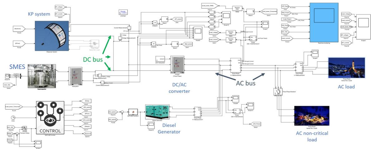
Figure 4.4: KP microgrid Simulink model
