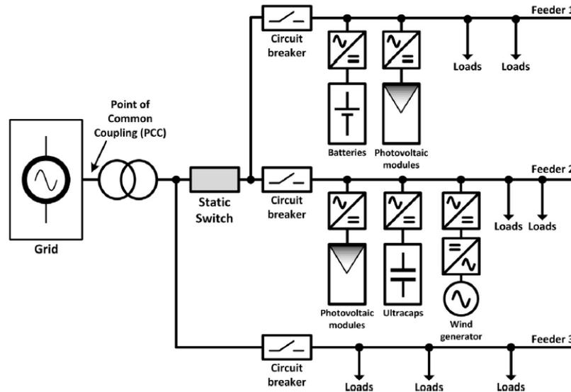
Figure 1.5: AC microgrid[18]
