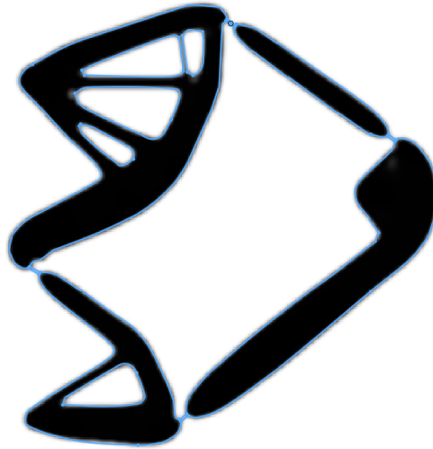
Figure C.2: Semi-automatically sketched balanced geometry in SolidWorks
