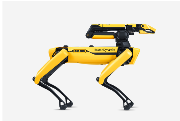
Figure 5-1: The Boston Dynamics Spot robot [2] equipped with an arm, turning it into a mobile manipulator. Mobile manipulation is essential in an urban SAR scenario that contains doors. The arm end-effector also contains a camera, allowing it to collect images in hard to reach places.
