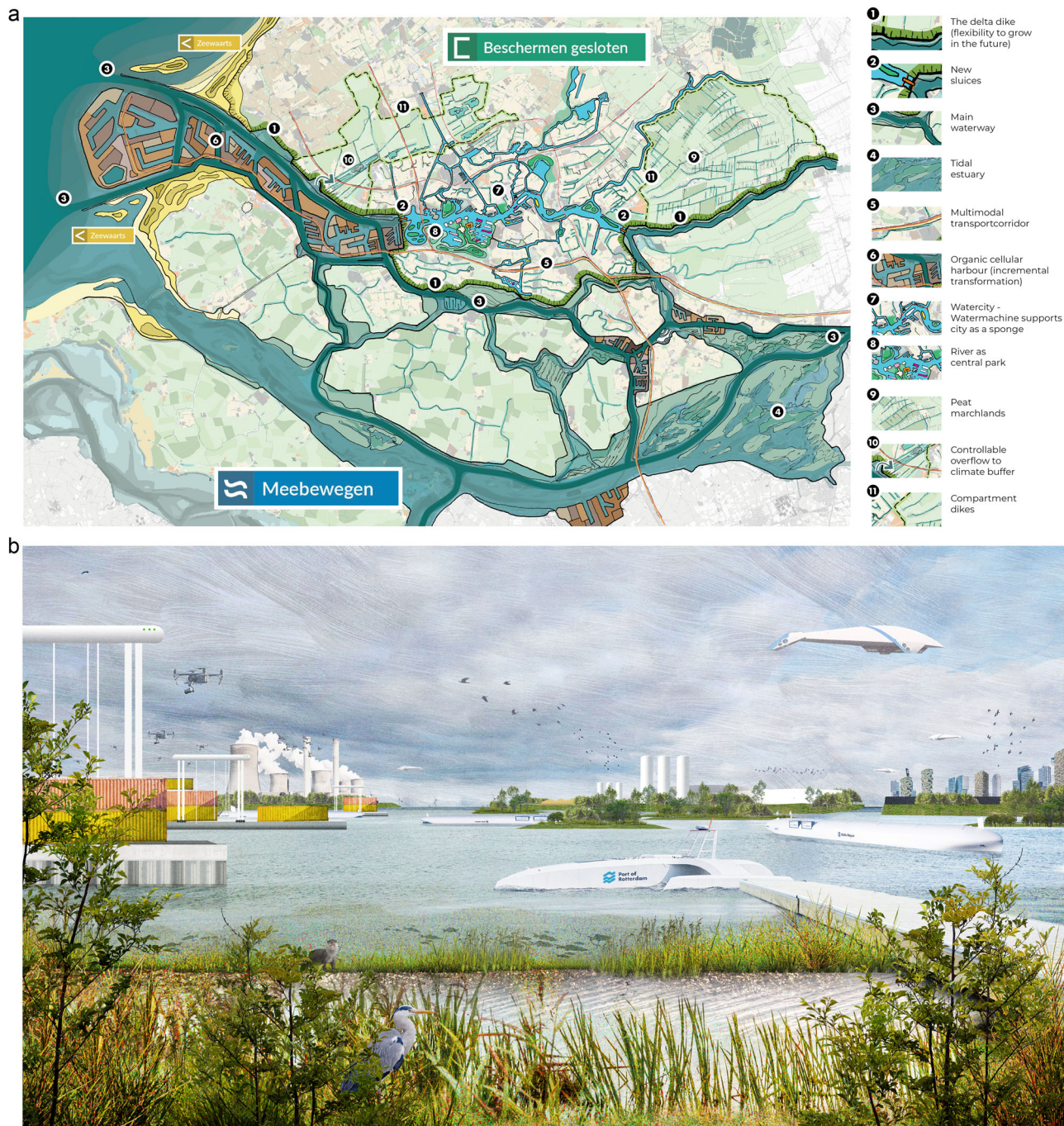
Fig. 2 | Envisioning the Dutch delta in 2022. Spatial design of a section of the Dutch delta (Fig. 2a) developed to protect the Port City area of Rotterdam. This will be achieved by rerouting the current flood defense (dike ring 14) and creating a sponge city. The port will continue to be elevated incrementally while simultaneously
