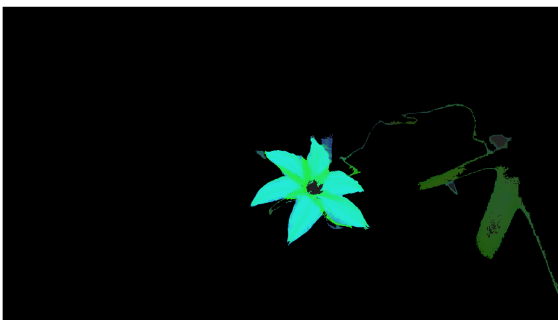
Figure 8.17: HSV image after performing closing by reconstruction
