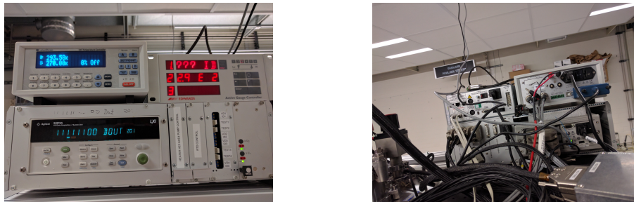
Figure 4.8: Control devices for the cryostat inside the laboratory. In the left: Agilent (green display) and Lakeshore (blue display) devices front panel. In the right: Rear side showing connections
