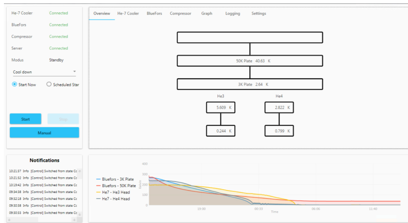
Figure 4.1: The GUI of the program as it can be seen on start up. The GUI consists of four frames: on the left upper side an information screen consisting of connection information and the ability to start and stop the system. On the right upper side a tab frame consisting of multiple views (see also figures below). On the left lower side a notification screen displaying important information, warnings or errors. On the right lower side a graph displaying temperatures of the Bluefors and He-7.
