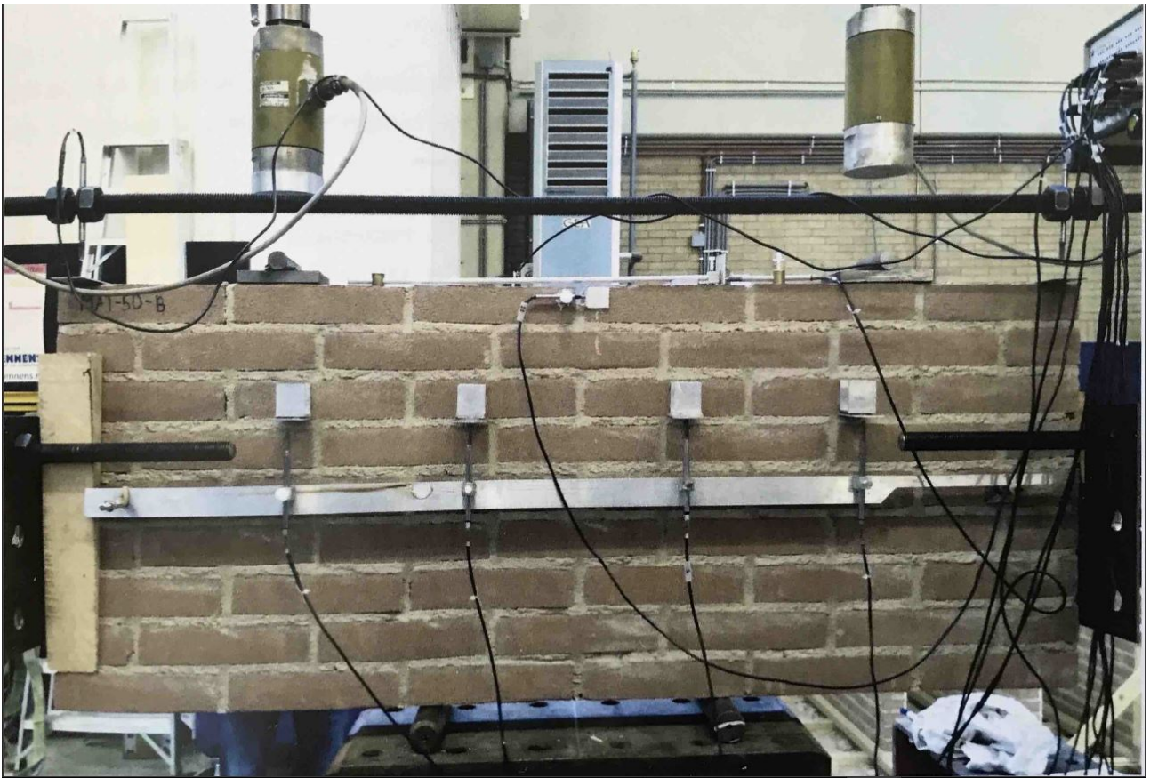
Figure 4.3: Window bank test sample (back side) [Korswagen et al., 2017]
