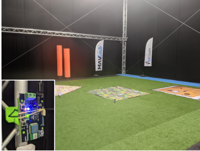
Figure 2.2: Flight data was collected in the "Cyberzoo" at TU Delft using a Crazyflie drone and the loco positioning system by bitcraze. Groundtruth is provided by an Optitrack motion capture system.
