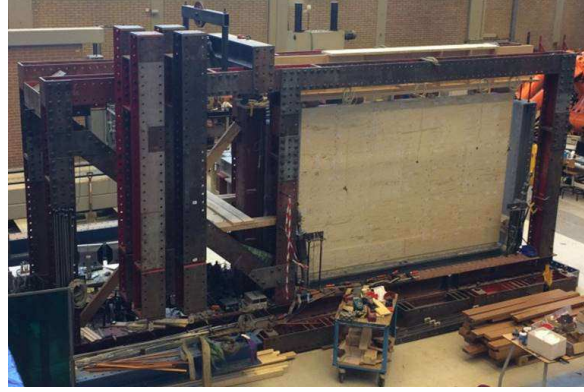
Figure 3: Setup for in-plane tests on timber diaphragms
