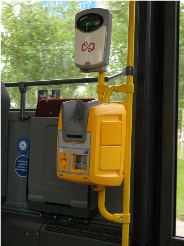
A Connexion onboard chipkaart fare reader with a debit card top-up machine underneath.
