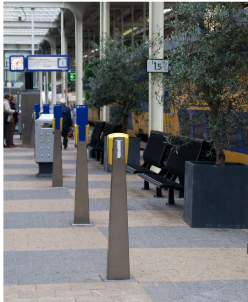
When two different rail operators call at the same platform, travellers must check in and out from each mode using the chipkaart readers of the respective operator. Here in Duivendrecht, the platforms have readers for both the NS national railways and the GVB metro.
