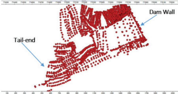
Figure 2.1: Point file of Lake Binaba created in saga from the XYZ text file
