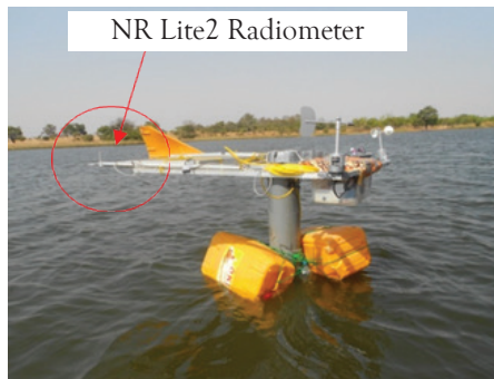
Figure 4.7: EC system on the 2nd floating Platform installed in the Lake Binaba with a NR Lite 2 Radiometer floating on a PVC pipe
