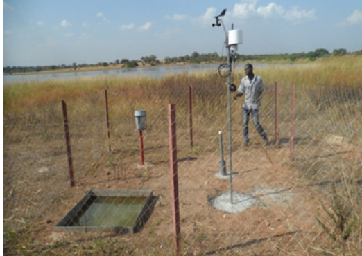
Figure 4.2 Colorado Sunken Evaporation Pan and an Automatic Weather Station set-up for Lake Binaba in the Upper East Region of Ghana
