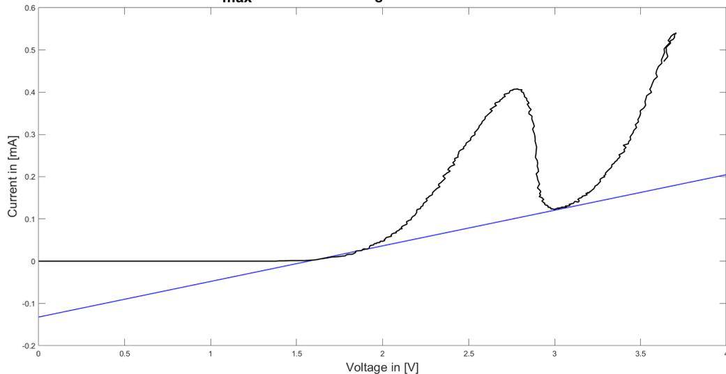
Figure 7.6: Smoothed voltammogram (time averaged over 20 ms) of  $60 \frac{\text{mmol}}{\text{l}} [\text{Na}^+]$  swept with  $V_{\max} = 2 \text{ V}$  and  $v = 1 \frac{\text{V}}{\text{s}}$  using a CNT-electrode, first wave with interpolation of baseline
