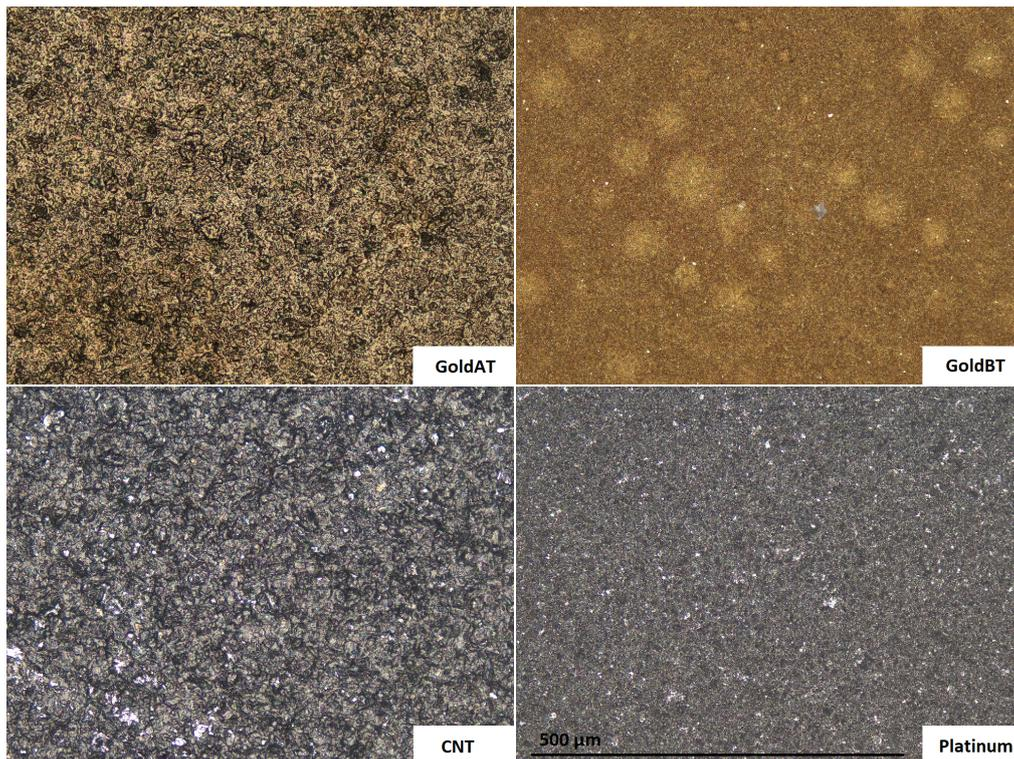
Figure 5.7: surfaces of active electrodes under 20x amplification top: two different gold surfaces; bottom left: CNT; bottom right: Pt
