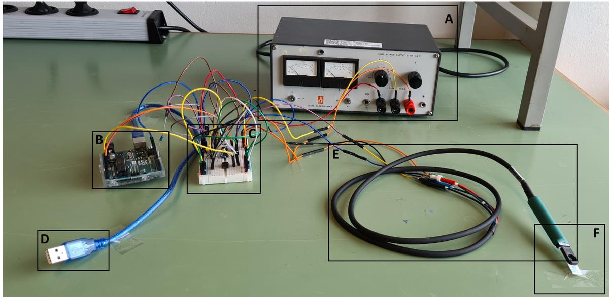
Figure 6.1: Implementation of voltammetric sweat sensor with (A) voltage source, (B) Arduino Microcontroller with ADC, (C) sensor electronics, (D) connector to laptop, (E) connector to electrode, (F) electrode
