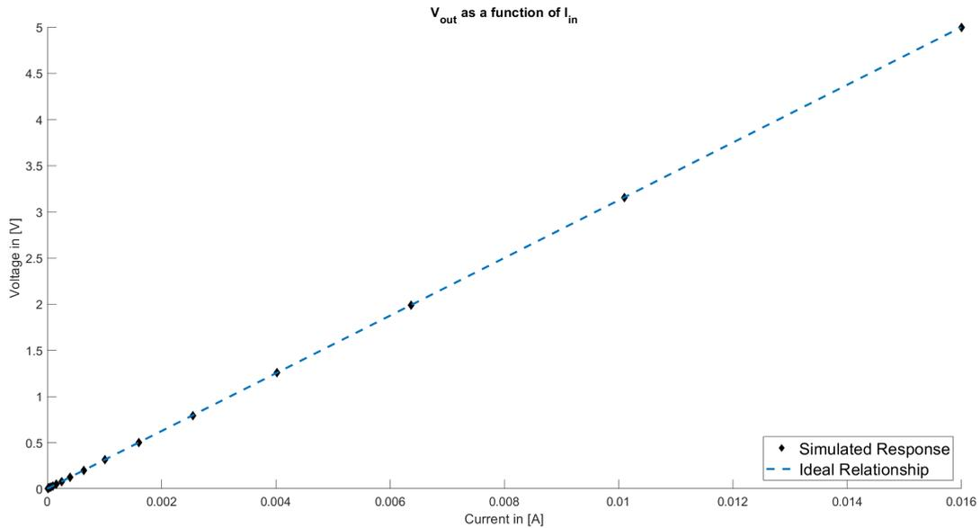
Figure 5.15: Output voltage over sweep of dynamic range of current (black) with ideal linear relationship (blue)
