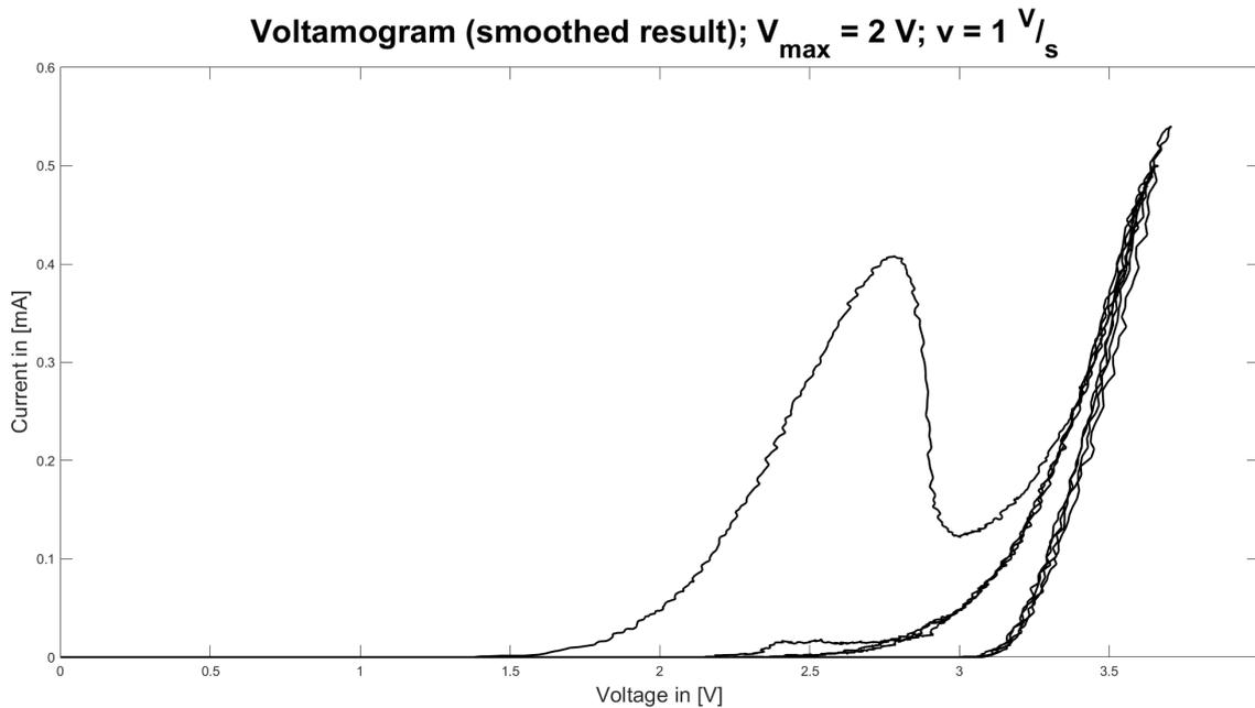
Figure 7.5: Smoothed voltammogram (time averaged over 20 ms, ionic current [mA] over CE-voltage [V]) of  $60 \frac{\text{mmol}}{\text{l}}$  [ $\text{Na}^+$ ] swept with  $V_{\max} = 2 \text{ V}$  and  $v = 1 \frac{\text{V}}{\text{s}}$  using a CNT-electrode
