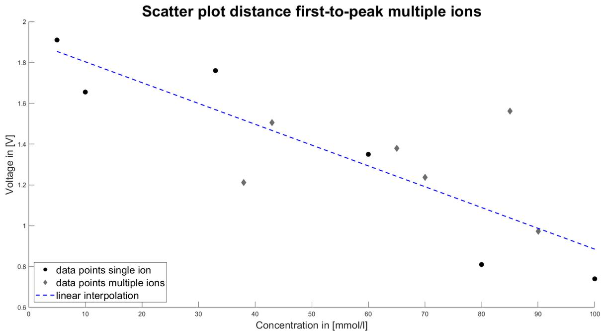
Figure 7.12: Distance between first current and peak location ionic solutions with different concentrations of sodium and potassium over the sum of concentration of sodium and potassium ( $R^2 = 0.73$  of the linear interpolation)
