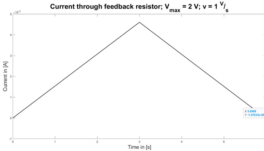
Figure 5.12: Overcurrent with purely resistive feedback after single sweep
