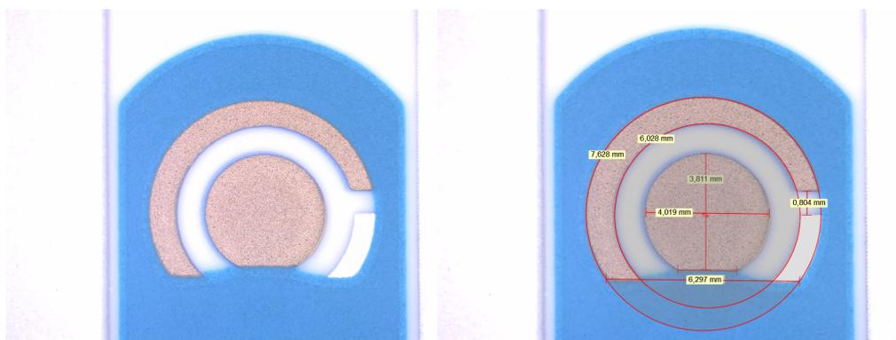
Figure 5.5: Pictures of the electrodes selected, left: without measurements, central WE with CE in ring around it (both platinum) and Ag/AgCl RE in bottom left corner; right: same electrode with detailed measurements for the accurate determination of surface area
