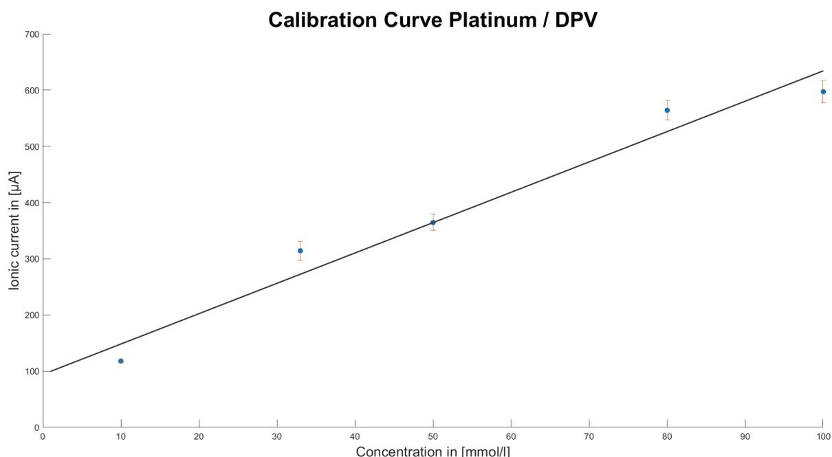
Figure 7.14: Calibration curve of DPV ( $R^2 = 0.934$ );  $V_{pulse} = 100\text{ mV}$ ,  $t_{pulse} = 100\text{ ms}$  and  $duty\ cycle = 50\%$  overlaid onto  $V_{max} = 2\text{ V}$  and  $v = 1\frac{\text{V}}{\text{s}}$ ; physiological concentrations of  $\text{Na}^+$
