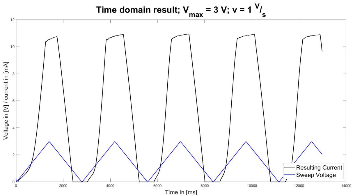
Figure 7.3: Dry test of voltage sweep with diode-load  $V_{\max} = 3\text{ V}$  and  $v = 1\text{ V/s}$
