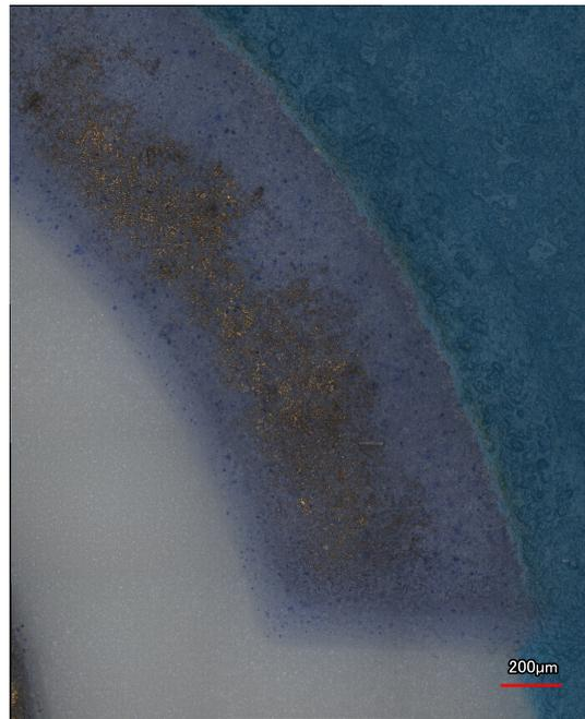
Figure 7.15: CE of gold electrode after stress test, 20x planar amplification
