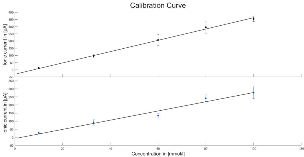
Figure 7.7: Calibration curve (linear approximation) of ionic current in  $[\mu A]$  over concentration of  $Na^+$  in  $[\frac{mmol}{l}]$  during calibration with ionic fluids of known concentration, with CNT ( $R^2 = 0.967$ ) in black, top and platinum ( $R^2 = 0.997$ ) in blue, bottom
