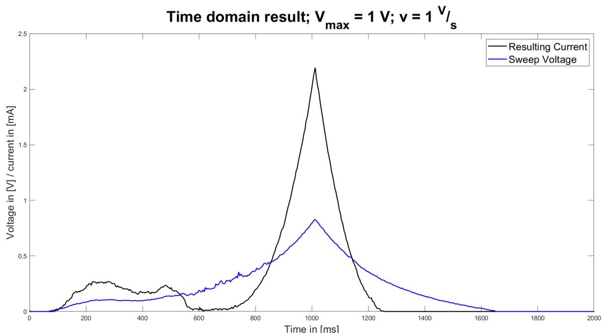
Figure 7.16: Time domain result of LSV with  $V_{max} = 1\text{ V}$  and  $v = 1\text{ V/s}$  of  $100\text{ mmol/l}$  [NaCl] and  $1\text{ }\mu\text{mol/l}$  [NaOH]
