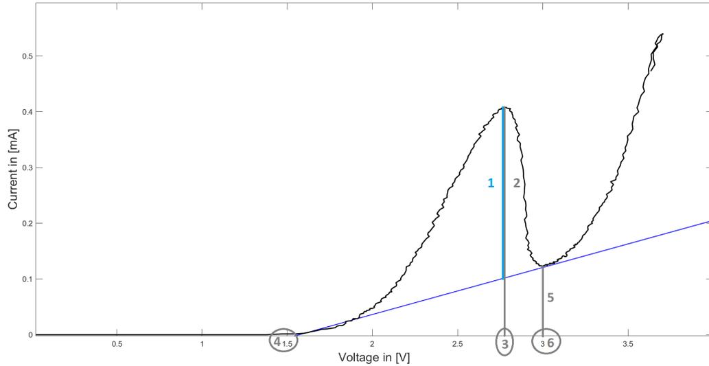
Figure 7.10: Typical voltammogram with curve features marked: (1) ionic current, (2) absolute peak height, (3) peak location, (4) first current location, (5) valley height, (6) valley location
