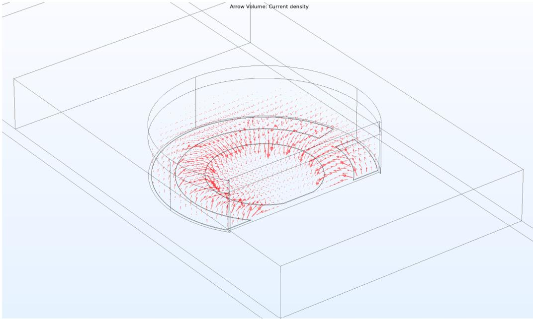
Figure 5.9: Current density after application of voltage step on CE and RE, length of arrow proportional to current density
