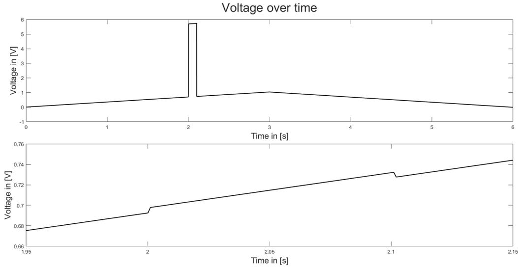
Figure 5.14: Ionic current induced between CE and WE superimposed on voltage sweep; ionic current modelled as pulse ( $t_{rise} = t_{fall} = 1\text{ ms}$ ,  $t_{on} = 100\text{ ms}$ ,  $I_{on} = 16\text{ mA}/16\text{ }\mu\text{A}$ ); plotted: (a) output voltage of TIA at  $I_{in} = 16\text{ mA}$ , (b) output voltage of TIA at  $I_{in} = 16\text{ }\mu\text{A}$
