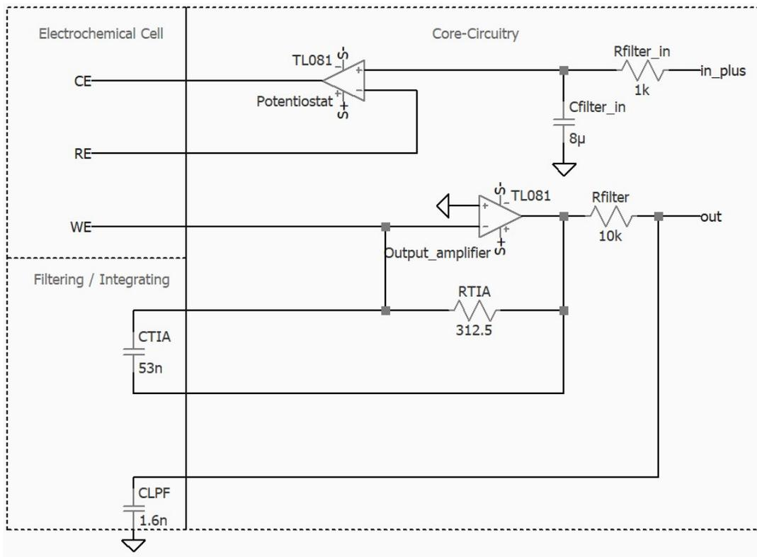
Figure 5.11: Full design of the sensor in LTSpice excluding PWM and ADC on Arduino for simulation of DR, linearity, SNR and WE stabilization
