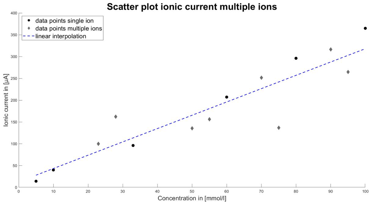
Figure 7.11: Ionic current of ionic solutions with different concentrations of sodium and potassium over the absolute difference in concentration between sodium and potassium ( $R^2 = 0.83$  of the linear interpolation)
