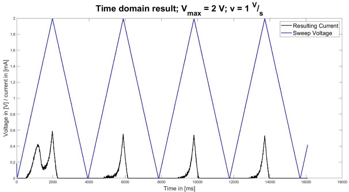
Figure 7.4: Time domain Sweep voltage and resulting ionic current of  $60 \frac{\text{mmol}}{\text{l}}$   $[\text{Na}^+]$  swept with  $V_{\text{max}} = 2 \text{ V}$  and  $v = 1 \frac{\text{V}}{\text{s}}$  using a CNT-electrode
