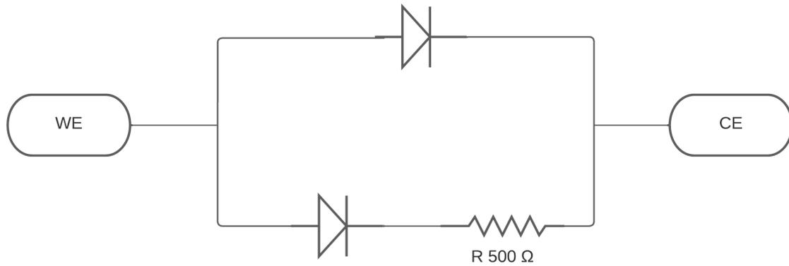
Figure 7.2: Schematic of dry test using diodes
