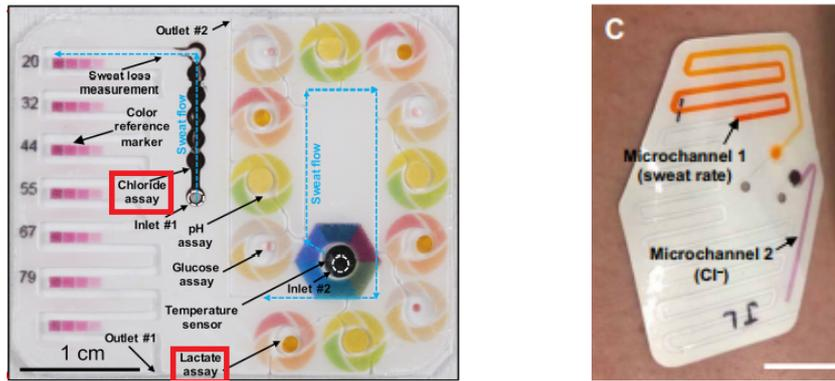
Figure 3.2: Different state of the art colorimetric sensors, left: full assay with the markers for fatigue highlighted, adapted from [40], right: collection system and colorimetric patch for  $\text{Cl}^-$ -measurement [46]
