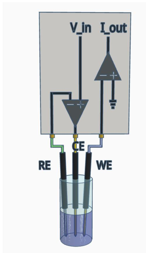
Figure 5.1: Basic setup of voltammetry with three-electrode-system submerged in sample and connected to potentiostat (electronics simplified)
