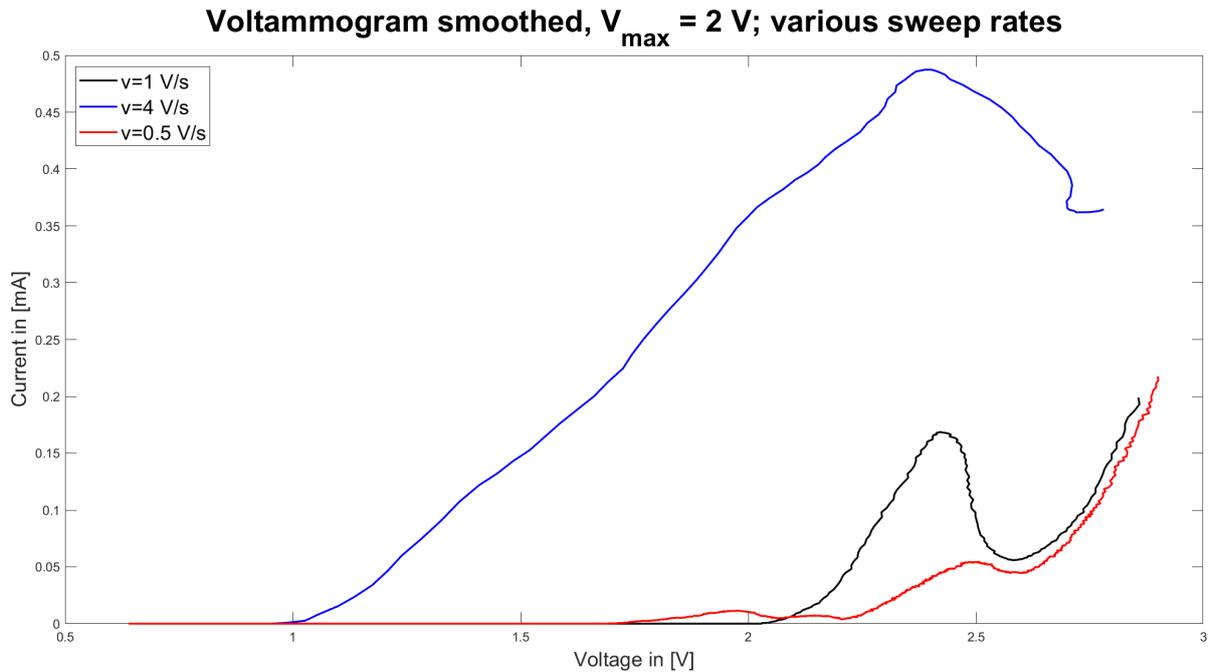
Figure 7.8: Smoothed voltammogram (time averaged over 20 ms) of  $100 \frac{\text{mmol}}{\text{l}}$   $[\text{Na}^+]$  at different sweep rates ( $v = 500 \frac{\text{mV}}{\text{s}}$ ;  $1 \frac{\text{V}}{\text{s}}$ ;  $4 \frac{\text{V}}{\text{s}}$ ); recorded with Pt electrode
