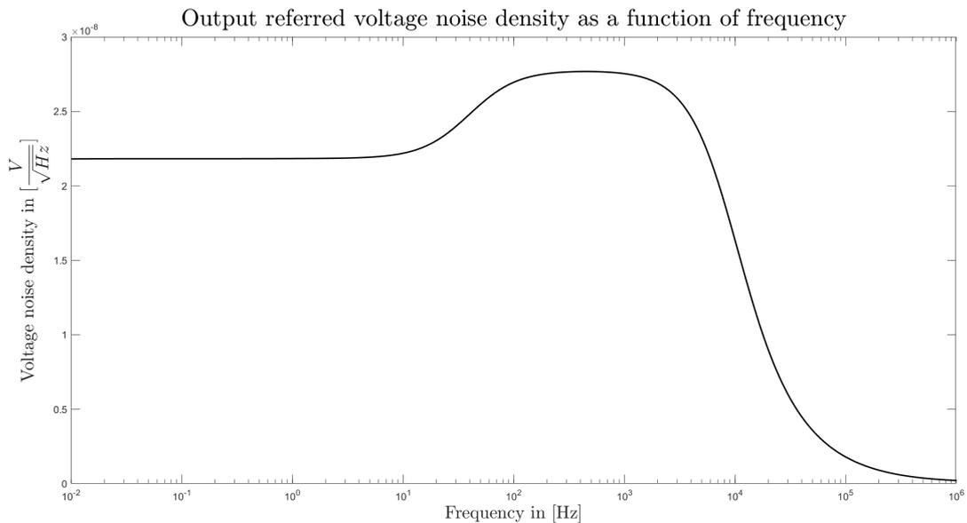
Figure 5.13: Output referred voltage noise of the system at in the frequency range between 10 *mHz* – 1 *MHz*
