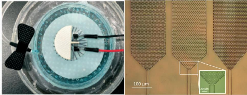
Figure 3.1: Different state of the art sweat collection mechanisms, left: fractal textiles emulating sweat patches [31], right: passive micro-pumps [32]
