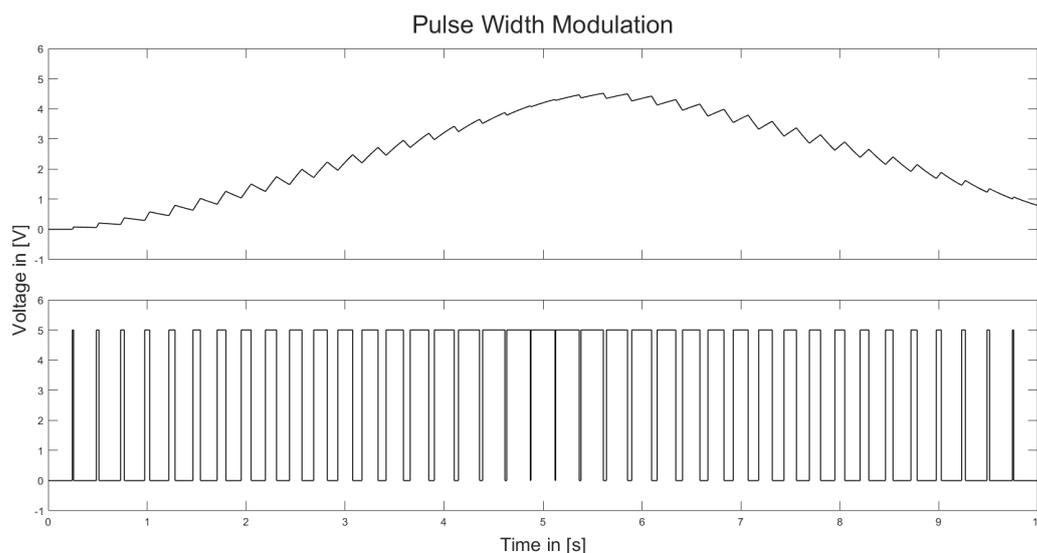
Figure 5.2: Principle of PWM with the resulting filtered signal at the top and the PWM signal at the bottom
