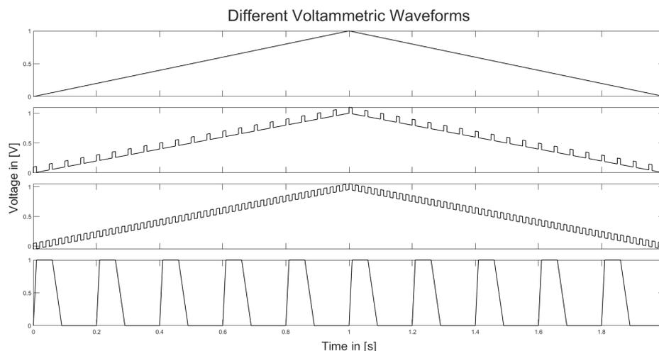
Figure 4.1: Different voltammetric waveforms sweeping from 0 to 1 V; from top to bottom: linear sweep voltammetry [LSV], differential pulse voltammetry [DPV], square wave voltammetry [SWV] and fast scan cyclic voltammetry [FSCV]
