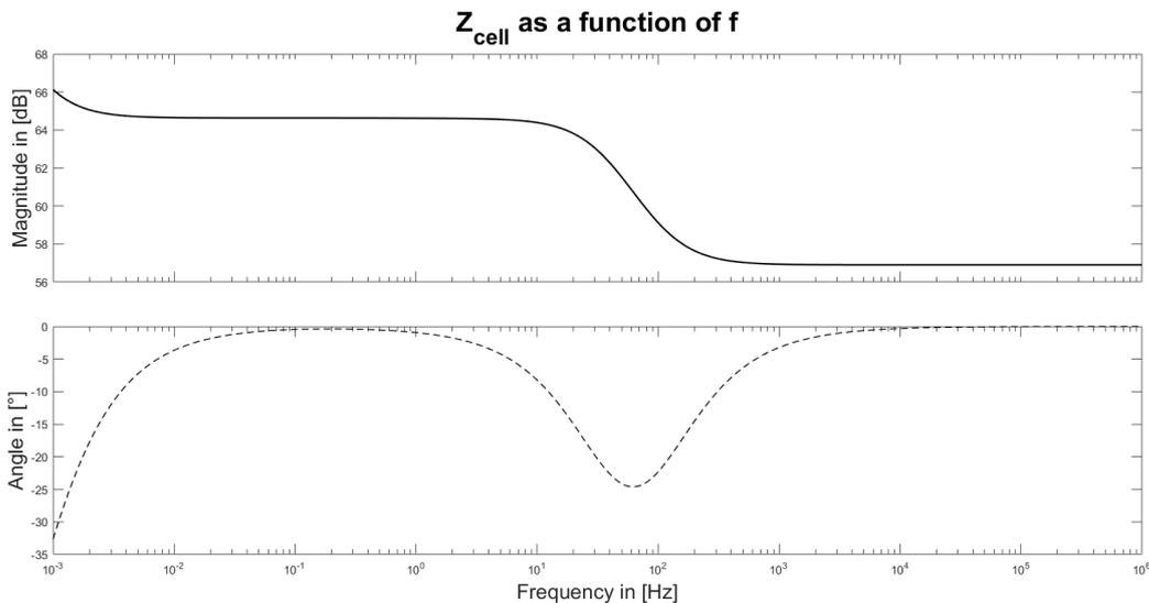
Figure 5.10: Bode plot of impedance of the electrochemical cell
