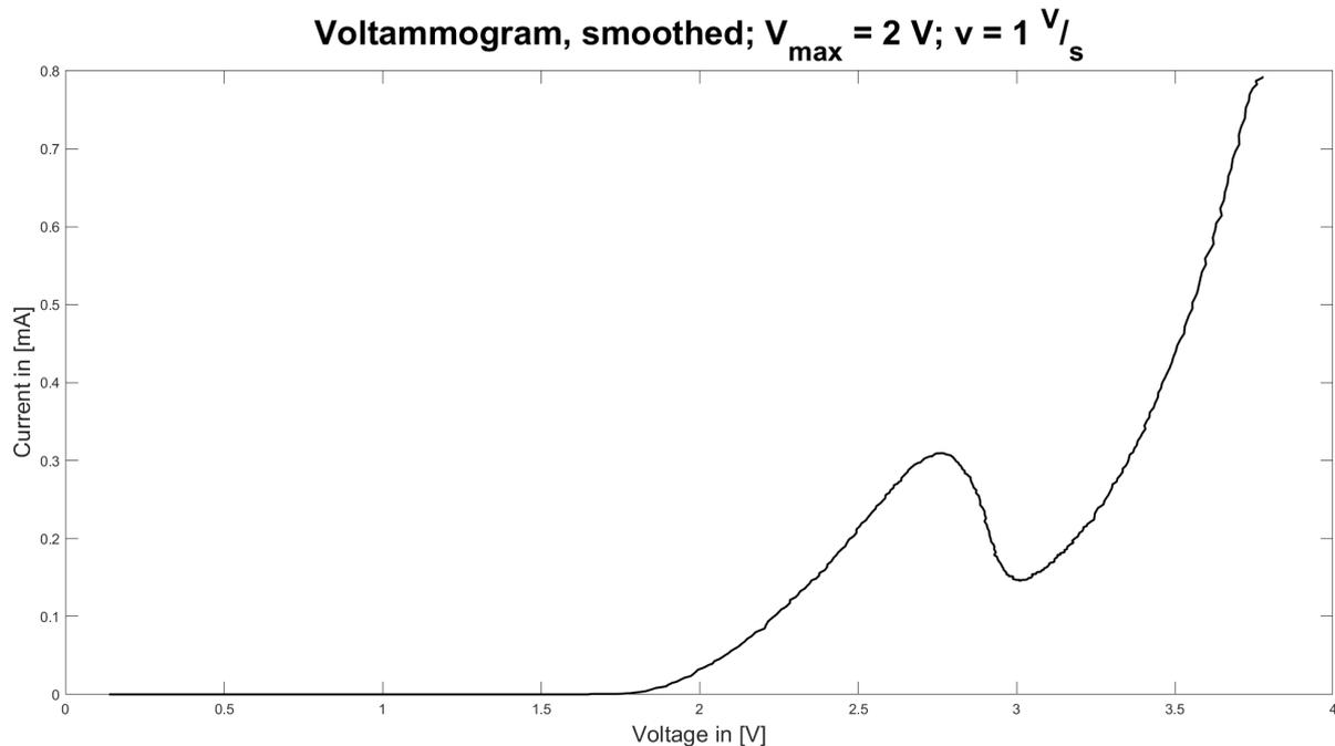
Figure 7.13: Smoothed voltammogram (time averaged over 20 ms) of real sweat collected during medium intensity exercise using CNT electrode;  $v = 1 \frac{\text{V}}{\text{s}}$  with a  $V_{\max} = 2 \text{ V}$
