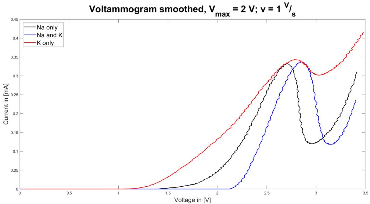
Figure 7.9: Smoothed voltammogram (time averaged over 20 ms) of linear sweep with  $V_{max} = 2\text{ V}$ ,  $v = 1\text{ V/s}$  of solutions with a concentration of  $100\text{ }\frac{\text{mmol}}{\text{l}}$  [ $\text{Na}^+$ ],  $10\text{ }\frac{\text{mmol}}{\text{l}}$  [ $\text{K}^+$ ] and a combination of both
