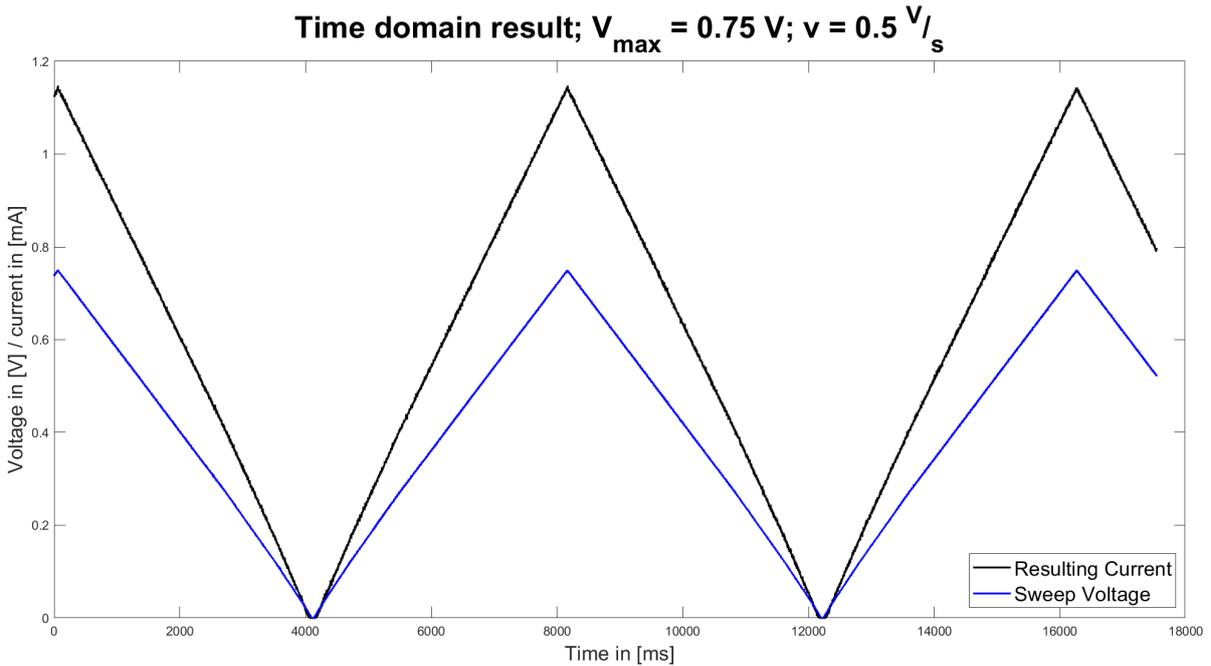
Figure 7.1: Dry test of voltage sweep with linear  $1,300 \Omega$  load,  $V_{max} = 0.75 \text{ V}$  and  $v = 0.5 \frac{\text{V}}{\text{s}}$
