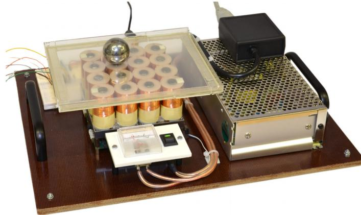
**Figure 2-3:** The planar magnetic manipulator setup. The ball rolls over a flat surface under the influence of the electromagnetic field generated by the combined action of 16 coils.
