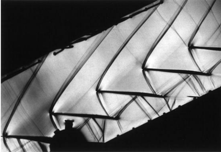
Figure 1.2: Schlieren image of SWBLI in compressor cascade at M=1.25 (Source: Institute of Propulsion Technology, DLR).
