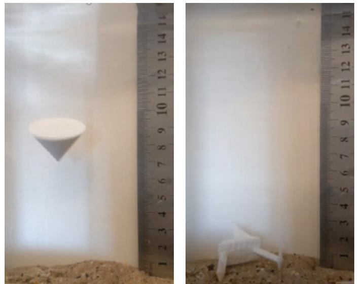
Figure 32: Two shapes during the sink test.
