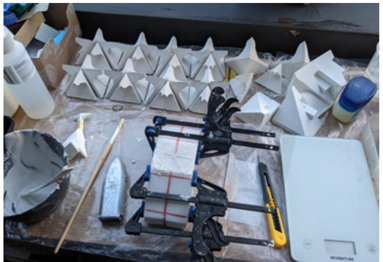
Figure 45: Casting of prototype in silicone mold.
