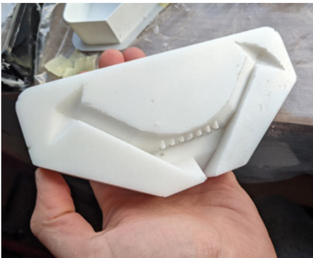
Figure 44: Silicone mold part.
