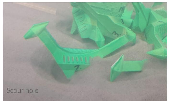
Figure 58 - 61: Prototypes on a sand bed in the flume.
