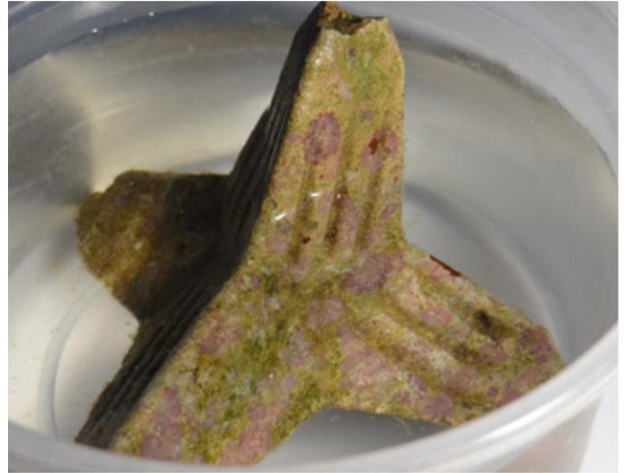
Figure 26: Biofilm on a concrete unit (photo: SECORE).
