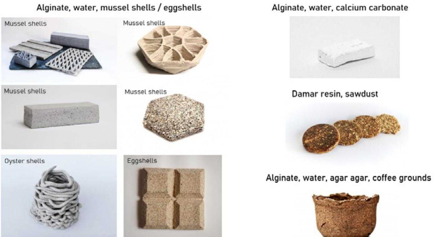
Figure 28: Examples of bio-based materials that could be suited.
