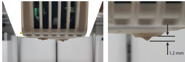
Figure 4.11 Ultimaker S5 printing head
