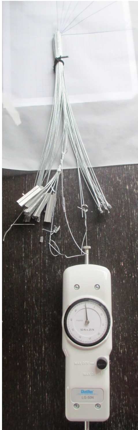
Figure 6.2: The test setup. The flexible shaft is shown with a black rubber band and the springs scale which is attached to one of the steering wire rope.
