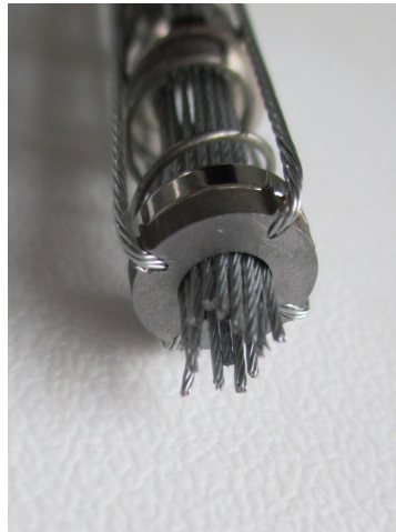
Figure 5.8: An isometric view of the flexible shaft with the tip and the four steering wire ropes included. Behind the tip a ring magnet and compression spring are shown which surround the inner wire ropes.
