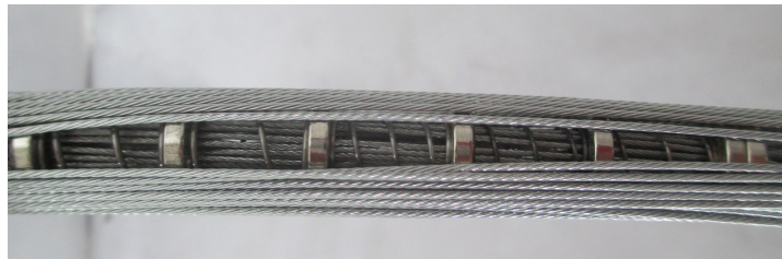
Figure 3.7: The prototype of the flexible shaft, which includes the inner and outer wire ropes, ring magnet and compression springs.
