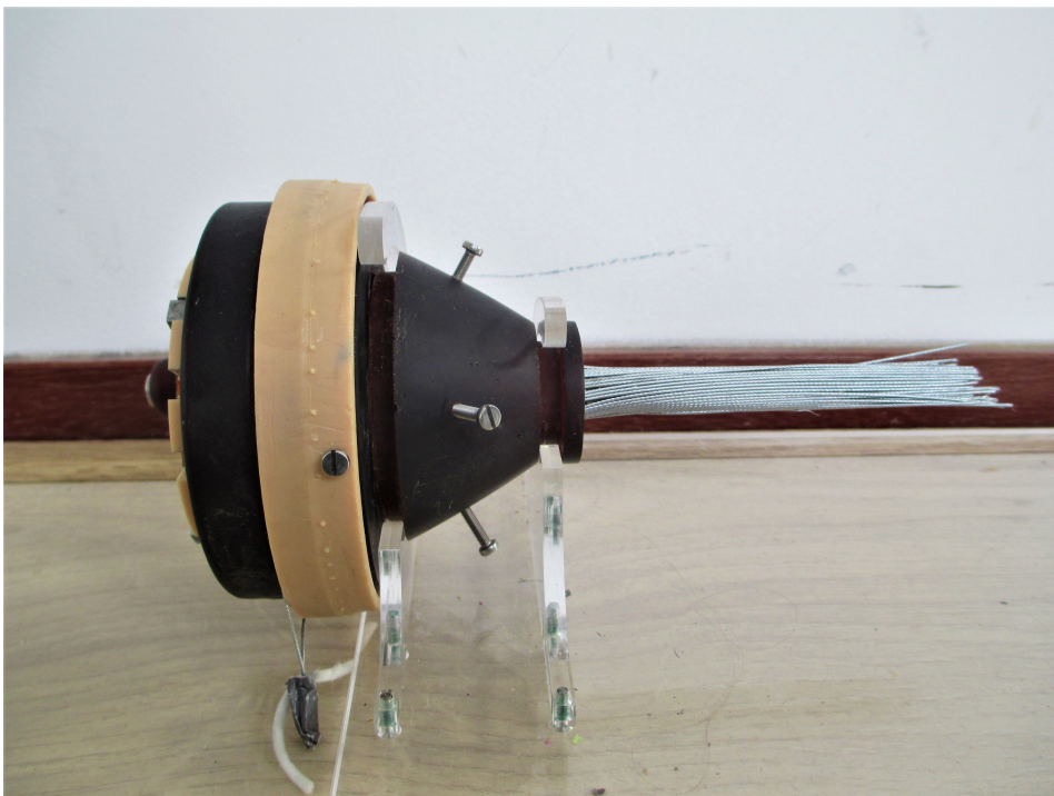
Figure 4.12: Side view of the actuation part of the prototype including the flexible shaft.
