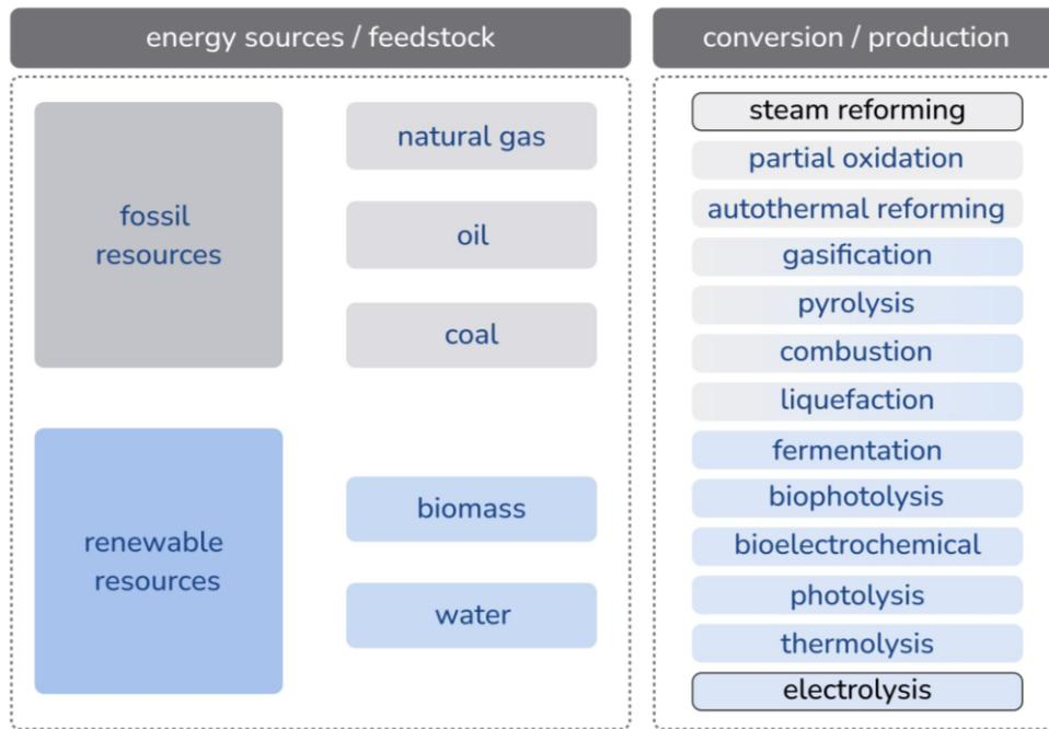
Figure 13 - Overview of various hydrogen production technologies
