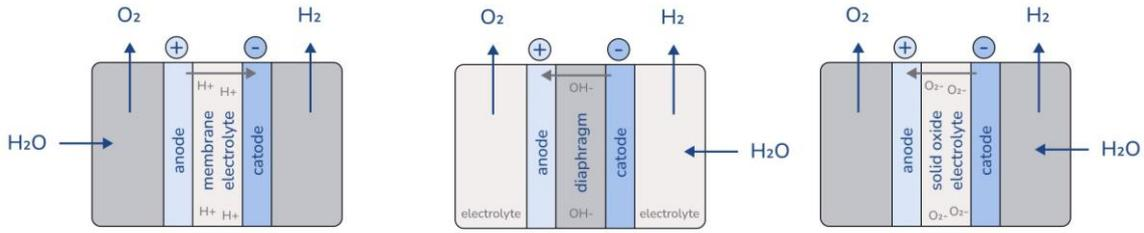
Figure 15 - Schematic of the main types of electrolyzers a) PEM b) Alkaline c) Solid oxide adapted from Araya et al. (2022)
