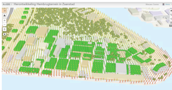
Figure 2: 3D visualisation of points in 3D space. These 3D points were used as source for the 2D contour maps of Figure 1. Source: ESRI
