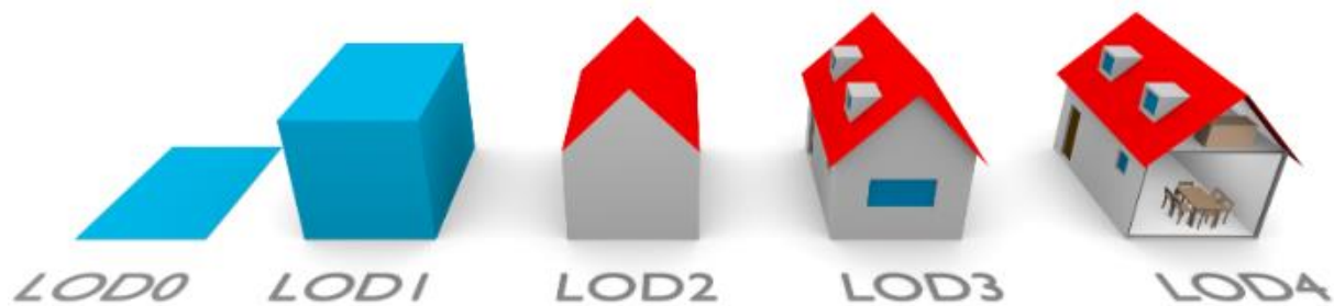
Figure 2. The five LODs of CityGML 2.0. The geometric detail and semantic complexity increase, ending with LOD4 containing indoor features (Biljecki et al., 2016)
