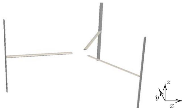
Figure 2: Top half of the VAWT as simulated in this work. To scale. Blades and struts are pitched as in Fig. 1.
