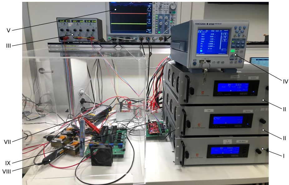
Figure 8.2: Picture of the experimental setup of the Interleaved TCM Buck converter in the lab. For the numbering of the equipment, see Table 8.1.
