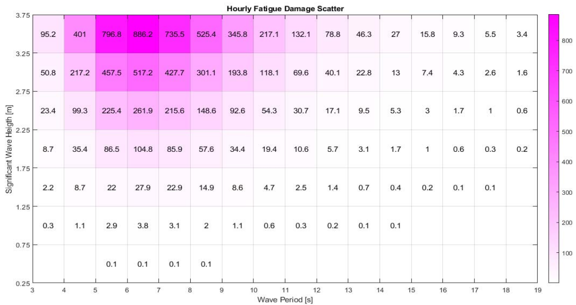
Figure 6.3: Hourly Fatigue Damage Scatter vs sea-state
