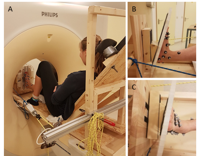
Fig. 2. Experimental setup with (A) the simulated weight-bearing device in the CT-scanner. Two examples of foot of foot plate positions: (B) medial view of the 20° dorsal flexion and (C) superior view of the 10° eversion.
