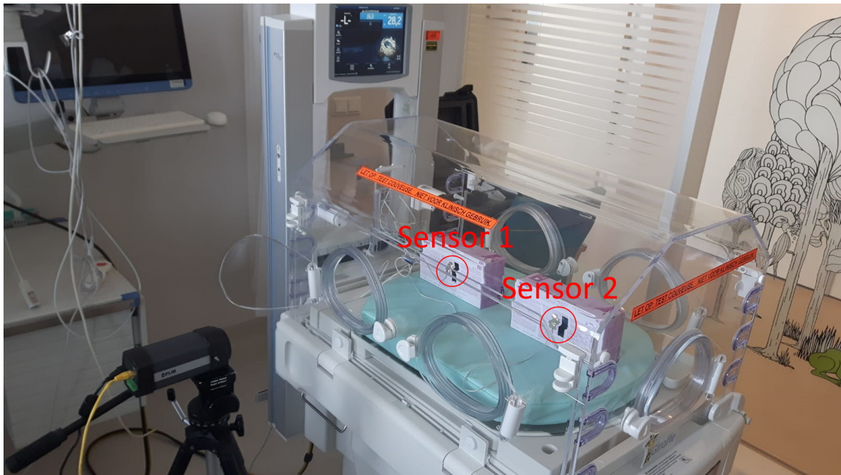
Figure 9.7: Measurement setup in RDGG during the measurement Opening Portholes . The box on the left was named Sensor 1, with the right box being named Sensor 2.
