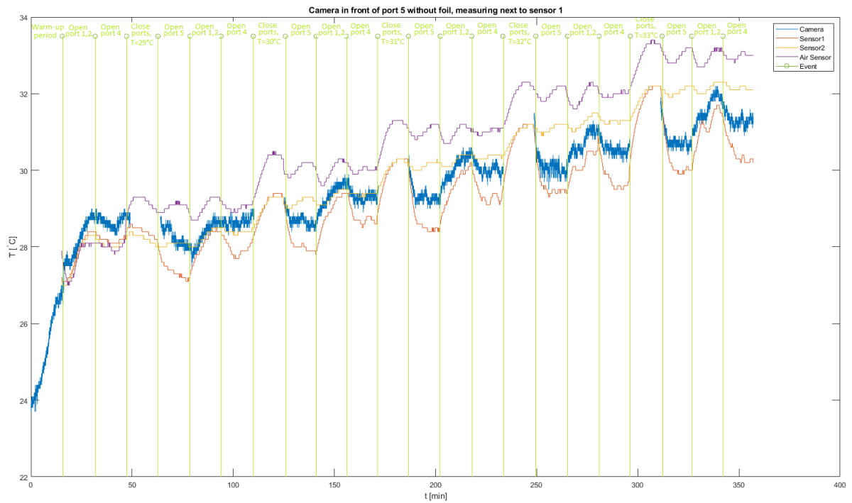
Figure 9.8: Visualisation of the effect of opening additional portholes on the temperature as measured by multiple sensors. The blue line depicts the temperature as measured by the IRT camera, the red and yellow line depict the values measured by the temperature sensors that are stuck to the paperboard boxes through hospital adhesives. The purple line represents the air temperature sensor, and the green vertical lines indicate an event.
