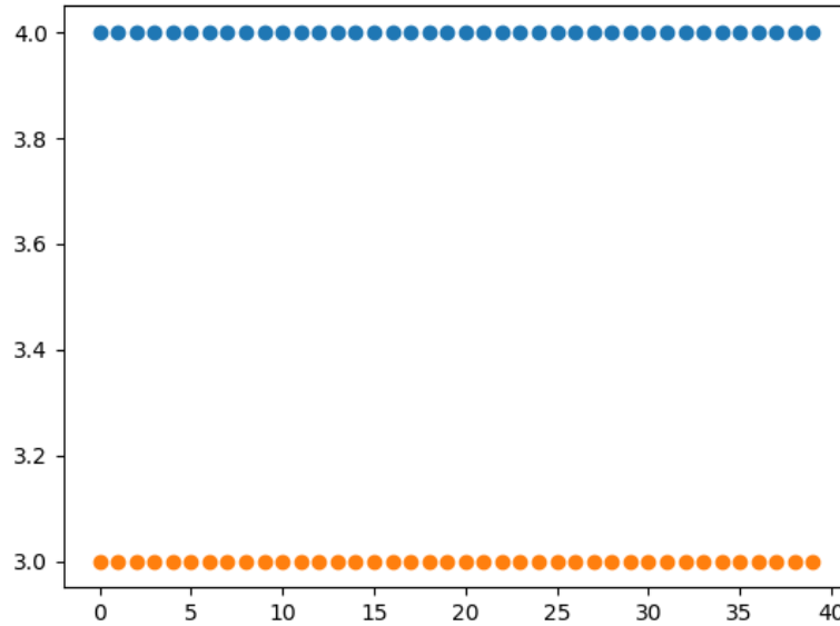
Figure 5.10: A graph on the number of iterations required for the standard Newton-Raphson iteration scheme to converge with a tolerance of \varepsilon = 10^{-5} versus i . The blue dots represent the standard problem, the orange the problem converted to a per-unit system.
