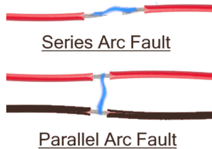
Figure 5.7: Arc faults as seen on wire level. [47]
