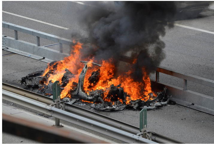
Figure 3.4: Damage done to a Tesla car after the battery underwent thermal runaway. [17].
