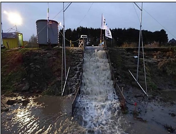
Figure 6. Observed aerated flow during the overflow experiment
