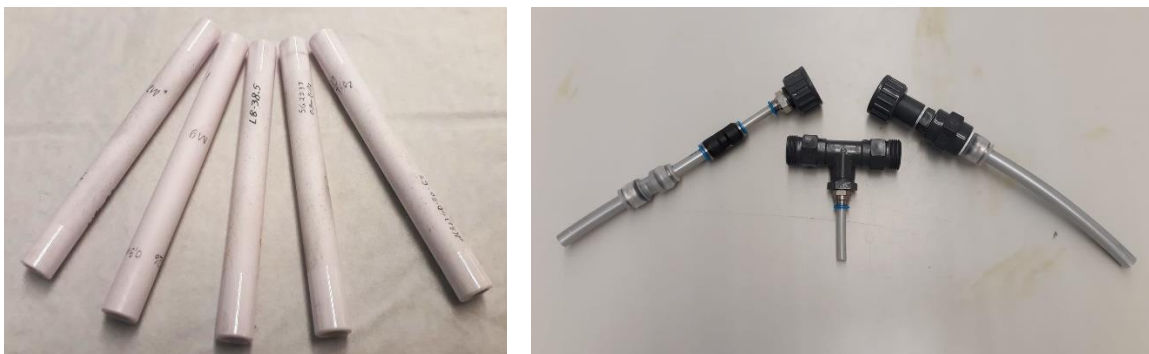
Figure 3.3. Ceramic NF membranes (left) and PVC module as the membrane housing (right)
