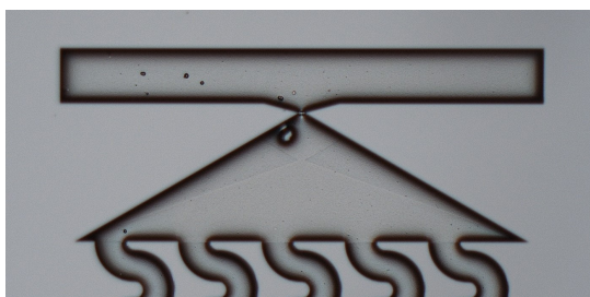
(a) W15R2C01 nozzle top-down view. Image captured with optical option of Keyence VK-X1000.
