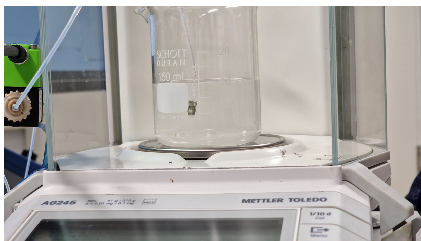
Figure 6.8: Detailed view of the exit tube in the beaker. The tube does not touch the sides or the bottom of the beaker, and its exit is fully submerged underwater.
