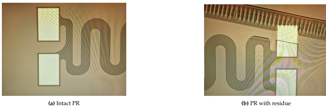
Figure 4.12: Comparison between intact heater photoresist, and photoresist with residue from coating.
