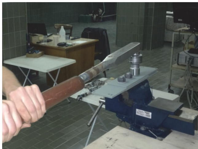
Figure 16. Bolt installation in specimens
