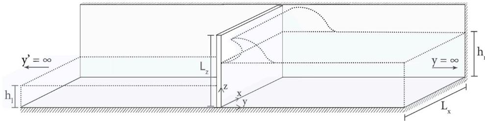
Fig. 1. Three dimensional overview of the plate model space.
