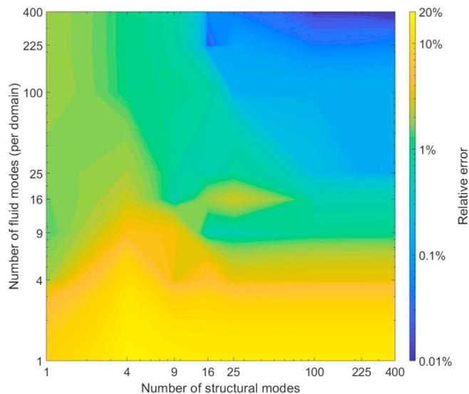
Fig. 12. The error in maximum plate stress found as a function of the number of structural and fluid modes taken into account relative to the result for both four hundred structural and fluid modes.
