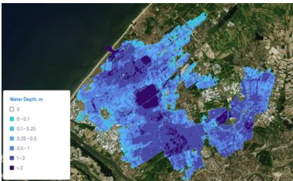
Figure 5.21: Inundation map of a flood event with a breach at Kijkduin. Based on a hydrodynamic simulation with a scenario of 1.5m sea level rise
