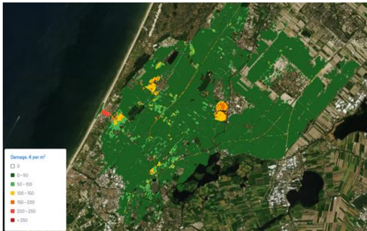
Figure 5.17: Map to indicate the estimated damages per square meter based on the hydrodynamic simulation for a breach in the dunes at Noordwijk.
