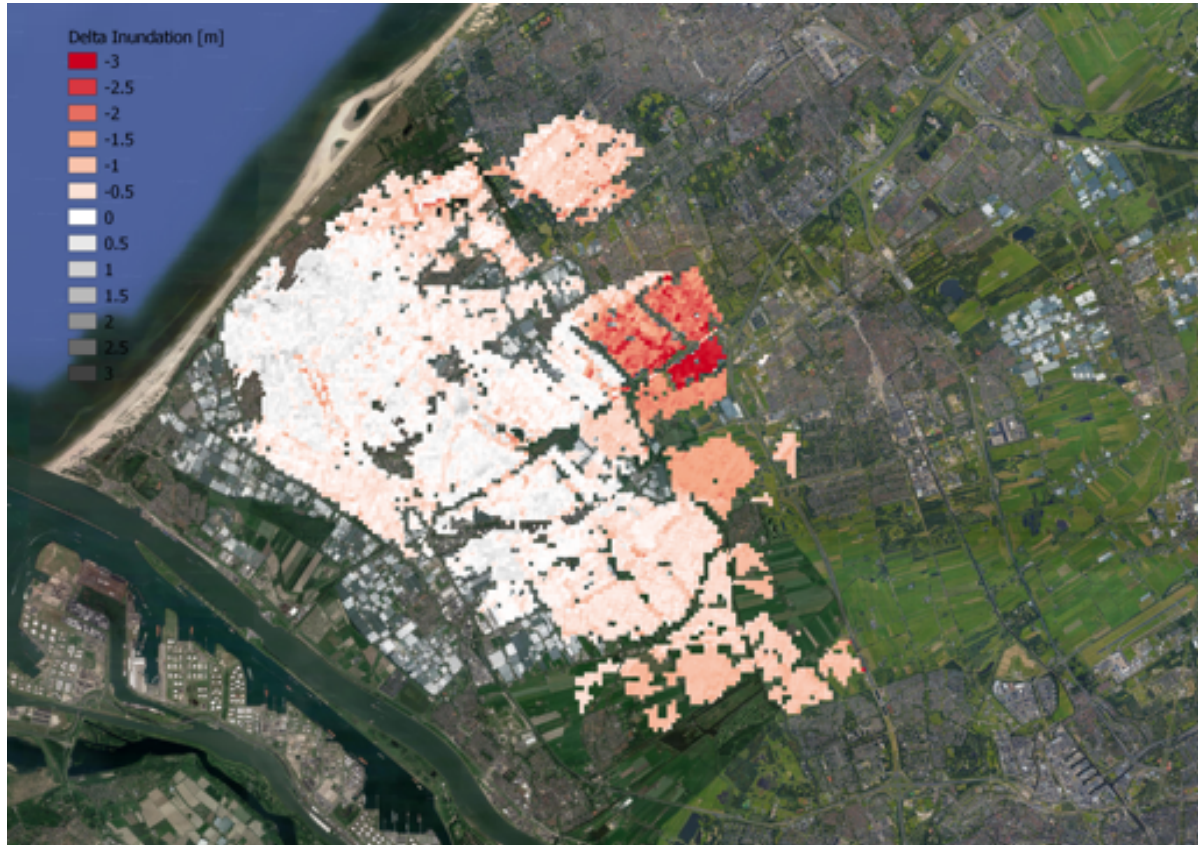
Figure 5.15: Map to indicate the difference between the inundation depths of the hydrodynamic simulation and the VNK2 for a breach in the dunes at Monster.
