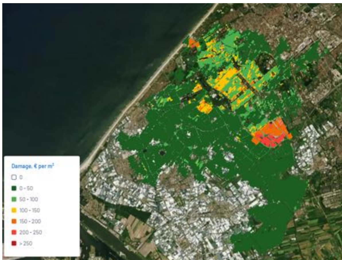
Figure 5.16: Map to indicate the estimated damages per square meter based on the hydrodynamic simulation for a breach in the dunes at Kijkduin.
