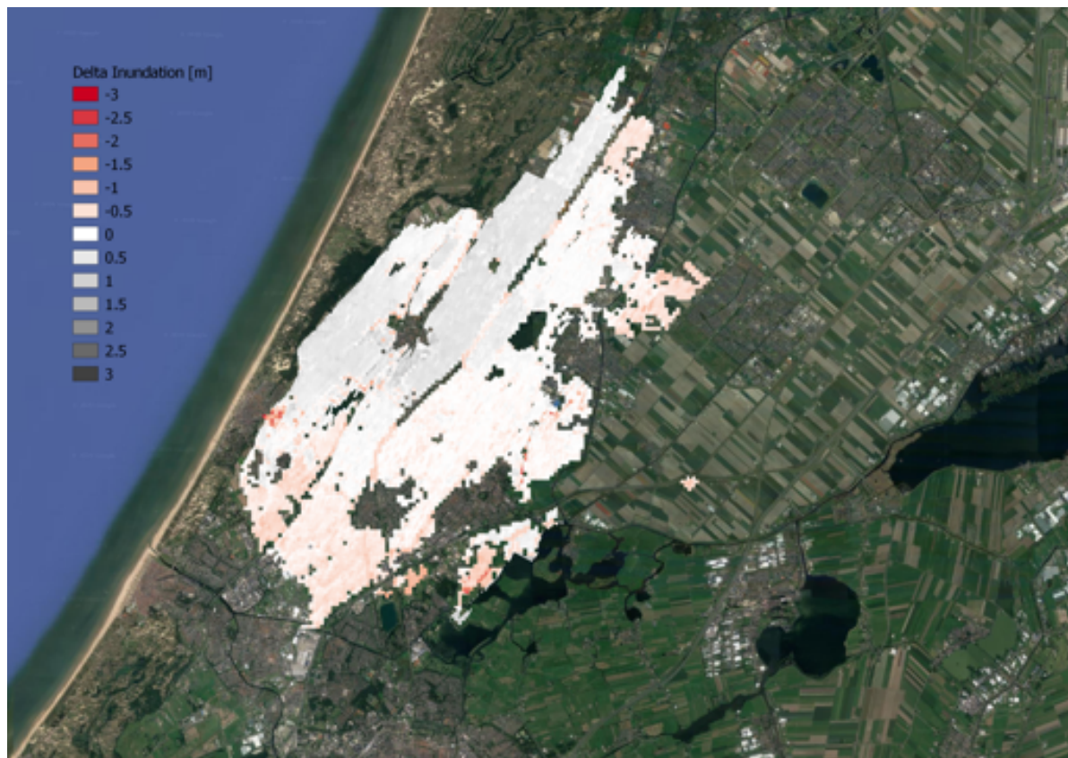
Figure 5.14: Map to indicate the difference between the inundation depths of the hydrodynamic simulation and the VNK2 for a breach in the dunes at Noordwijk.
