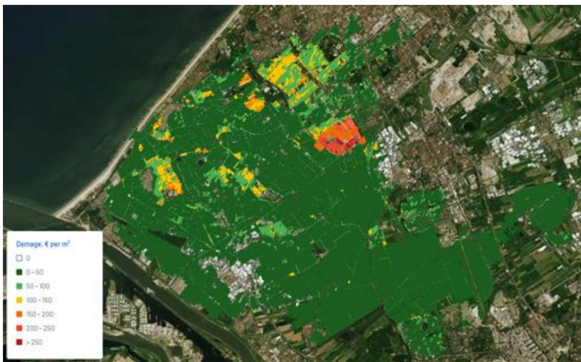
Figure 5.18: Map to indicate the estimated damages per square meter based on the hydrodynamic simulation for a breach in the dunes at Monster.
