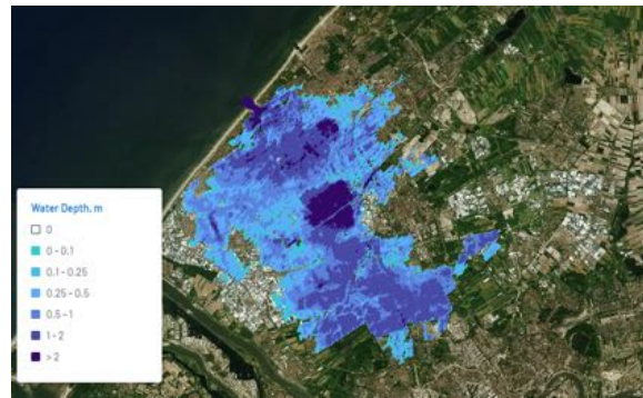
Figure 5.20: Inundation map of a flood event with a breach at Kijkduin. Based on a hydrodynamic simulation with a scenario of 1.0m sea level rise
