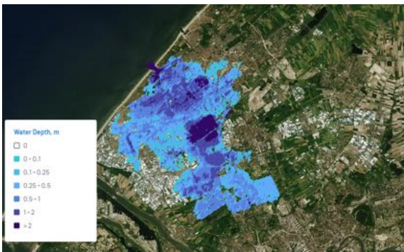
Figure 5.19: Inundation map of a flood event with a breach at Kijkduin. Based on a hydrodynamic simulation with a scenario of 0.5m sea level rise
