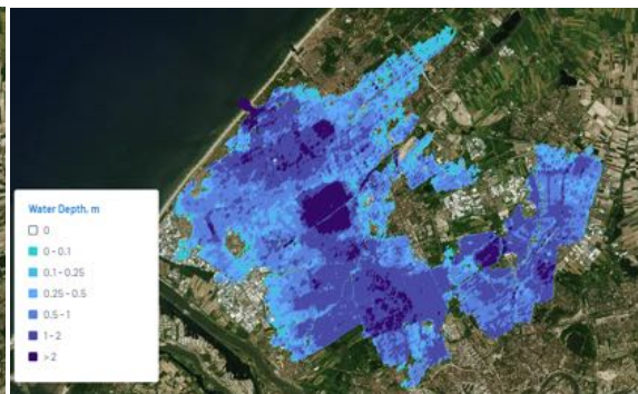
Figure 5.22: Inundation map of a flood event with a breach at Kijkduin. Based on a hydrodynamic simulation with a scenario of 2.0m sea level rise
