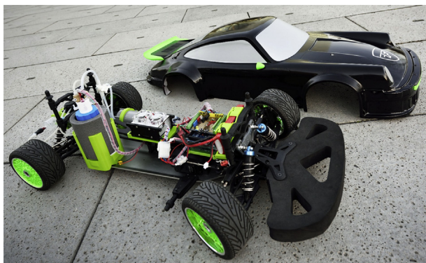
Fig. 2 – Formauto Junior: proof-of-concept 25 W model car for testing and marketing purposes.
